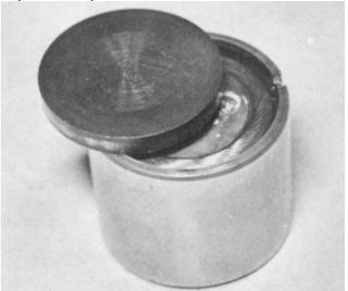
3.49B ... prise out the vlave clearance adjusting shim
