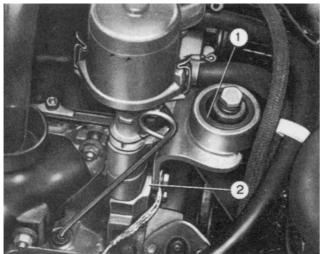
Fig. 13.4 Engine mounting (right-hand side) (Sec.3)
