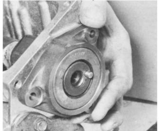
3.53 Fit the camshaft seal in its carrier to the cylinder head.
