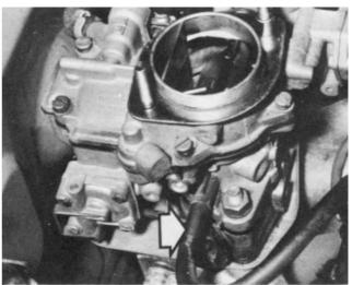
4.5 Weber single venturi carburettor installed (vacuum pipe arrowed
