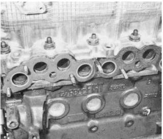
3.93A The two-pieces gasket for manifold joint...
