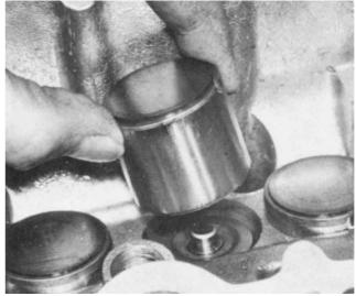
3.49D Refit each tappet bucket with its shim to its vlave
