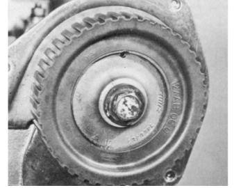
3.56 Fit the camshaft toothed pulley
