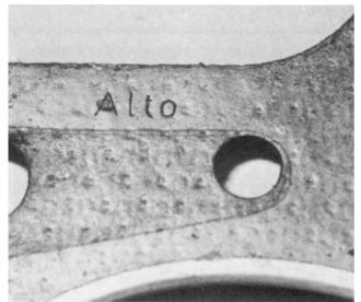
3.60 The cylinder head gasket is fitted ALTO upwards
