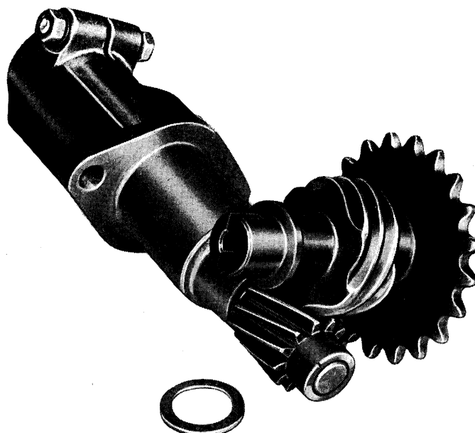
Fig. 79. - 118 B.000 engine ignition distributor-oil pump drive gear set and shaft, with thrust washer.
