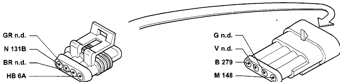
325 Connection bewteen injection/left front cables (1998)
