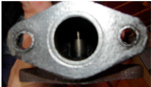
Now take the hose and attach it on the EGR valve. And with your mouth suck in the air out of it. When you sucked enough the valve will open. Do it a few times so the valve can work it self in.
