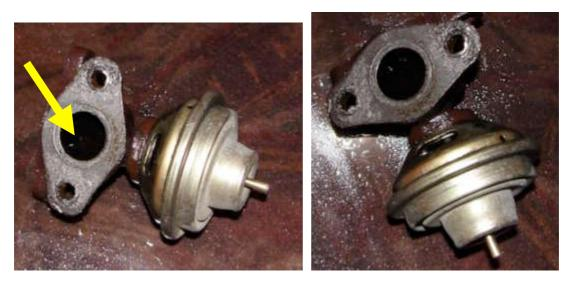
Fill the hole pointed with a yellow arrow and leave it to soak about an hour.
