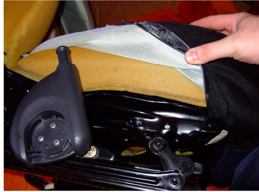
You may now have noticed that there are three metal rods running the whole length of the lower cushion and a strut rod near the front of the cushion (Shown as red lines). The yellow arrows point to metal ring clips that need to be removed. These ring clips hold the rods within the cover to a metal rod within the foam cushion. Whatever you do, do not cut the metal rods. Only the metal ring clips. Work your way left to right in a row removing the clips, try not to bend the metal rods in the cover.
