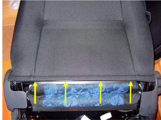
Lift the flap up to reveal a plastic clip. This clip hooks onto another clip. This is where the back facing of the cover meets the front facing cover and is held in place.
