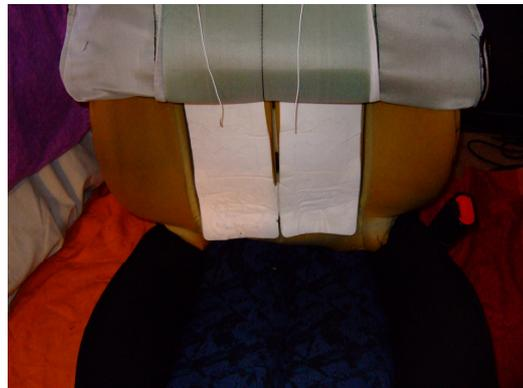
For those with the heated seats you may want to remove this. Whilst I was removing mine, it was lifting off a small layer of the cushion as well, so make sure this is kept to a minimum. Take your time and be patient. Use a hair dryer to soften the glue and/or use a sharp knife.
