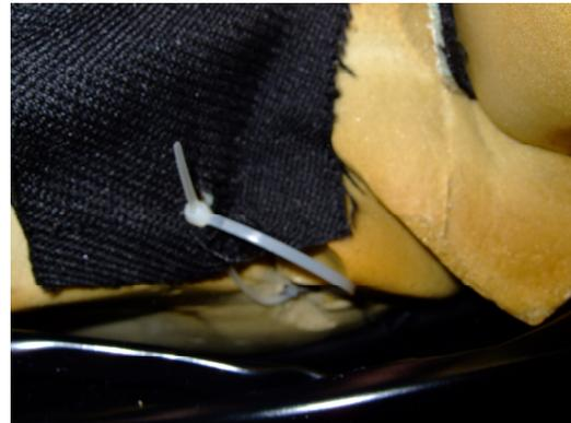
Reattach the cover to the sides of the seat, they basically fold over and push back in. You will hear them clip into place. Once complete feed the cover between the lower and upper cushion, make sure you don't trap any of the wiring and then reattach the clip to the bottom of the seats frame.
