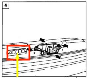
On this element that is on the car chassis, near the lock hinge. You need to clean the square plates with a fine sand paper. Yellow arrow.
