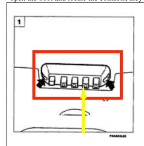
On this element that is on the boot, you have to clean the tips of the contacts. Pointed with a yellow arrow. To do it, use some fine sand paper.
