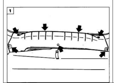
To get the access to the earth wire you must remove this. It's the boot plastic lid on the chassis of the car.
