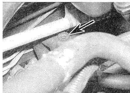
31.27 Bleed screw (arrowed) on heater hose
