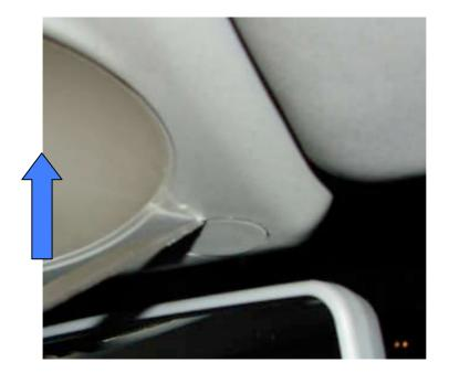
You do it by taking a knife or a small flat screwdriver and you pull it off by pushing the knife in the arrow direction.
