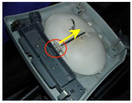
After you have the light free. Take off the white plastic lid by pressing the red circled point in the arrow direction and pulling it upwards.
