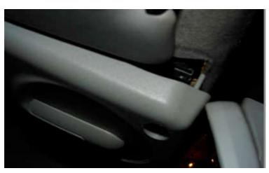
Then after you have removed the plastic covers off, you will see two screws in the holes. Unscrew these out and pull the light will fall off like in the pic. Then just pull it off.
