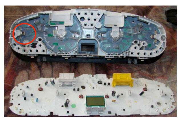
slightly move the pins (circled red on the above pic) in the direction of the arrow.
