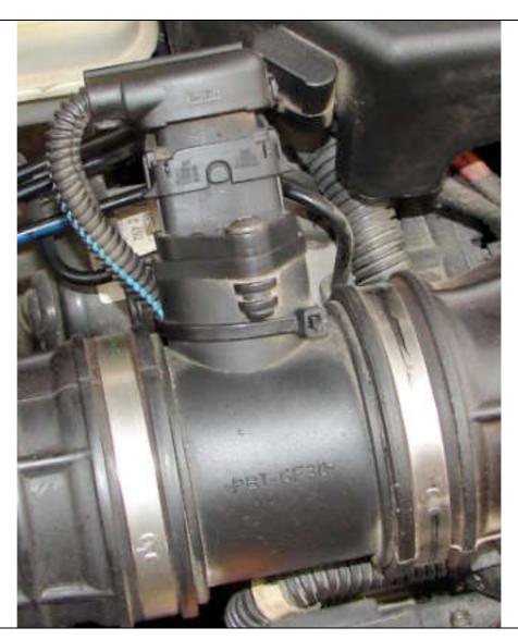
The second step is to unplug the connector on the MAF sensor. It has a clip that holds it firmly in place, so you need to push the clip with your finger to release it. (red arrow) Then just pull the plug off.
