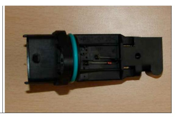
The next step is the cleaning. For that you will need a 3 or 4 cotton sticks and some alcohol. \*Use clear alcohol or start spray – do not use any spray or liquid that is oily or greasy.
