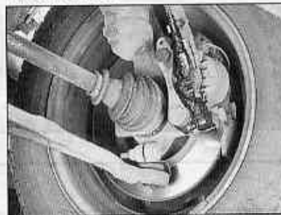
A leak occurring at a wheel is almost certainly brake fluid.
