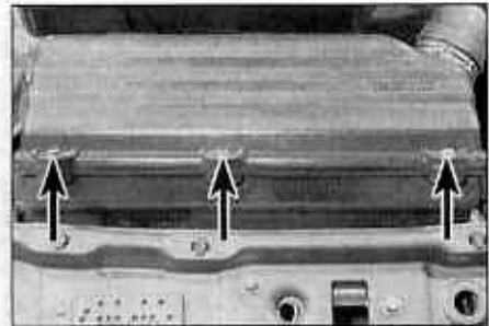
18.6 Undo the three bolts (arrowed) and disconnect the air cleaner cover rear retainers (16-valve engines)
