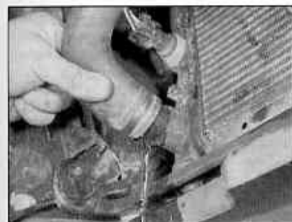
27.2 Disconnecting the radiator bottom hose to drain the coolant
