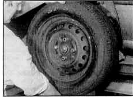
12.4 Rocking a roadwheel to check for wear in the steering/suspension components
