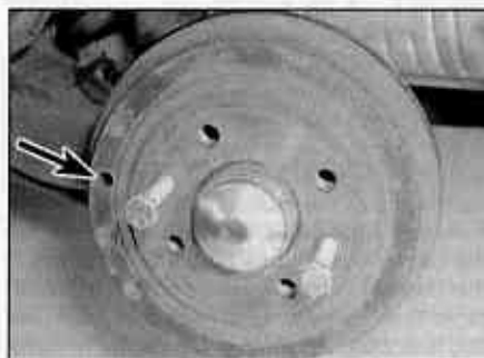
29.2 Check the thickness of the shoe friction material through the hole on the edge of the drum (arrowed)
