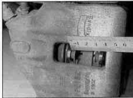
6.2 Check the thickness of the pad friction material through the hole on the front of the caliper
