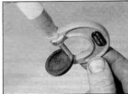
18.13 Measuring the thickness of a shim using a micrometer
