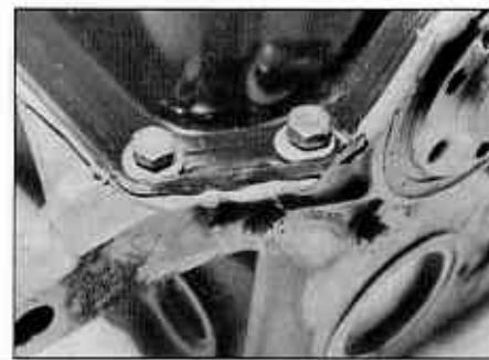
12.5b Sump fixing screw and flange end fixing nut
