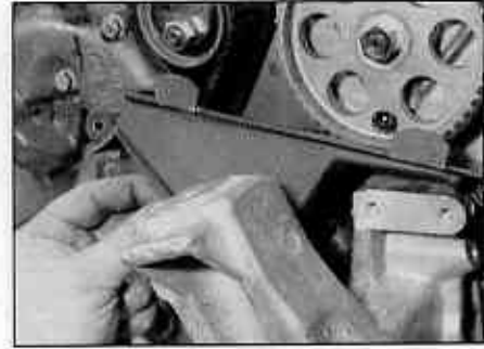
2.13 Removing the lower timing cover
