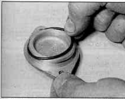
9.22a Locate a new O-ring on the inlet camshaft cover plate . . .
