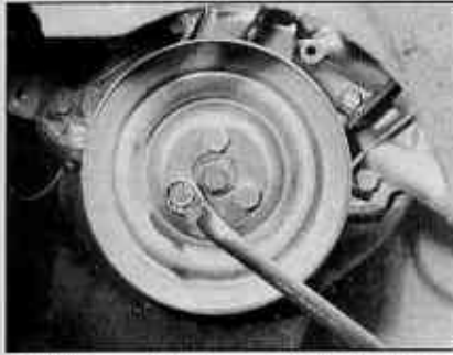
2.11 Unscrewing the crankshaft pulley bolts
