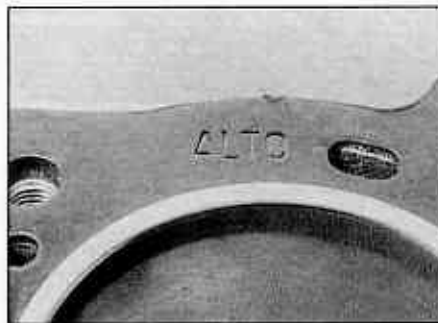
9.22b . . . so that the ALTO marking can be read from above
