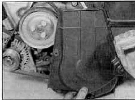
2.11 Removing the outer cover over the crankshaft pulley
