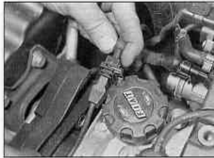
4.11b ... then slide the wiring plug and socket from the timing cover slot
