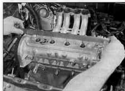
4.22 Place a straight edge along the top of the rods and turn the crankshaft until the straight edge contacts all four rods
