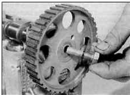
5.20a Unscrew the camshaft sprocket securing bolt and washer . . .
