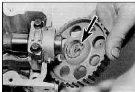
5.20b . . . and slide the sprocket from the end of the camshaft. Integral location key (arrowed)
