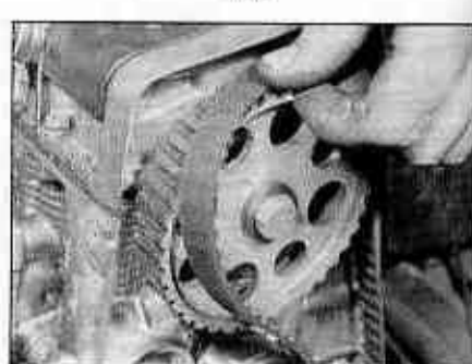
4.15 Fitting the timing belt
