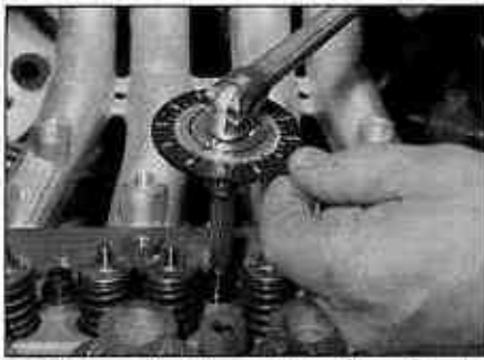
10.20c ... then through the Stage 2 and Stage 3 angle
