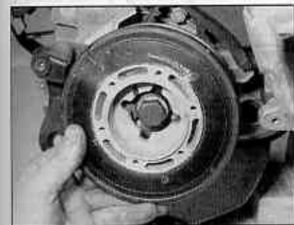
2.14b ... and remove the pulley from the front of the crankshaft
