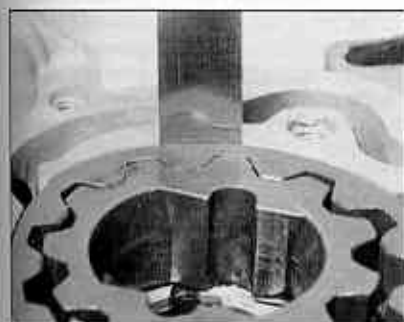
13.10a Measuring oil pump outer gear-to-pump housing clearance
