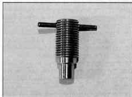
2.6a To make an alternative camshaft locking tool ...
