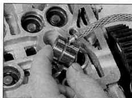
9.24 Lubricate the cam followers and place them in position in their respective bores
