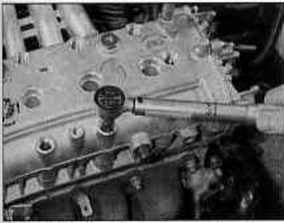
8.12 Refit the cylinder head extension retaining bolts and tighten them to the specified torque
