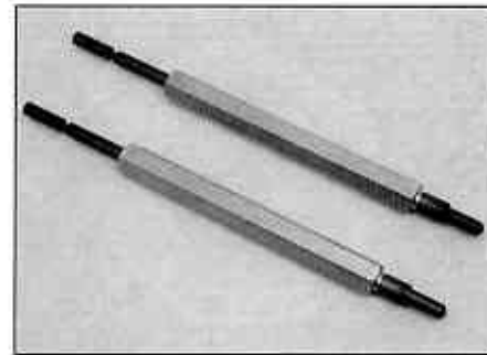
2.2b Fiat special tool for setting piston position ...
