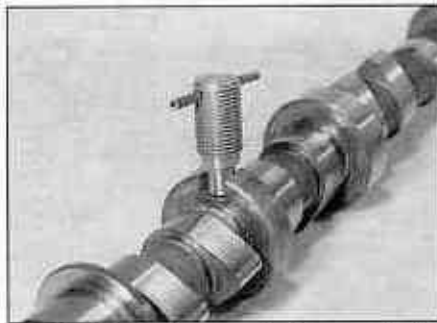
4.24b The tools engage in the camshaft slots when fitted (shown removed for clarity)
