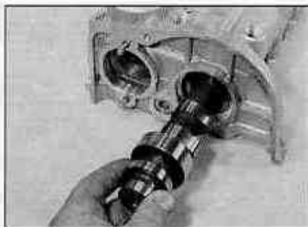
9.11 ... then remove the exhaust camshaft from the cylinder head extension
