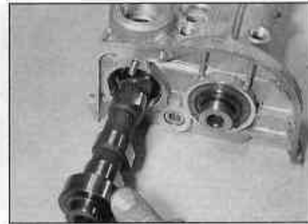
9.9 Carefully remove the inlet camshaft from the cylinder head extension
