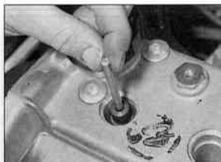
4.21c ... then insert the dowel rods
