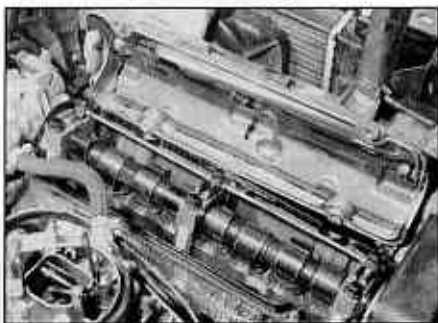
6.2 Removing the camshaft cover
