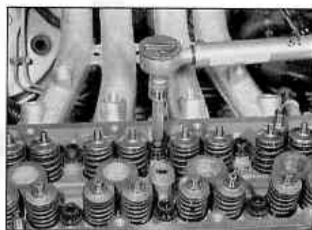
10.20b Tighten the cylinder head bolts to the Stage 1 torque setting . . .
