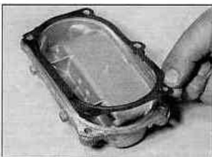
9.20a Locate a new gasket on the cylinder head extension end cover ...
