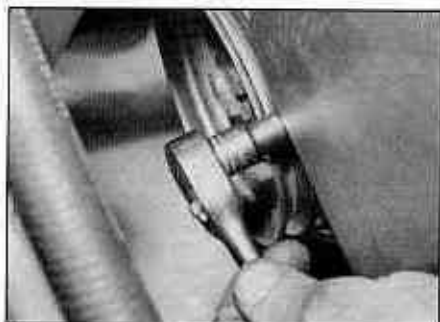
4.7 Removing the timing belt cover bottom bolt
