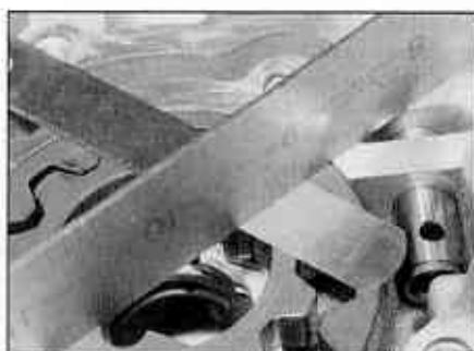
13.10b Measuring oil pump gear endfloat
