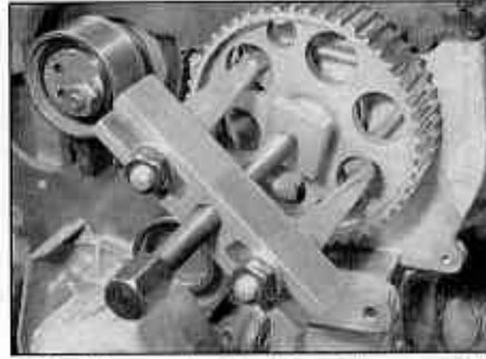
5.31a Use a puller to release the sprocket from the injection pump shaft
