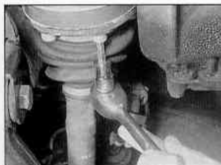
4.62a Use an Allen key to unscrew the inner driveshaft bolts
