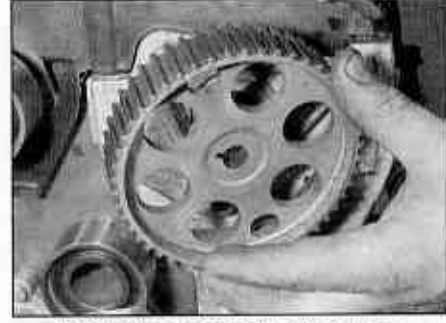
5.31b Remove the injection pump sprocket ...
