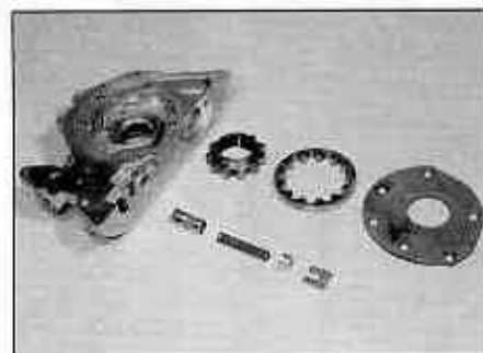
13.9e Oil pump housing and components
