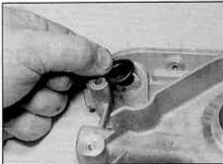
13.15 Engine oil dipstick rubber grommet in the oil pump casing
