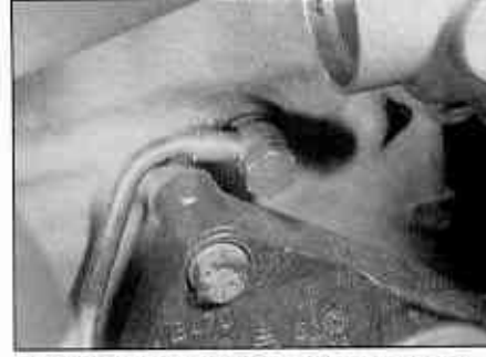
9.16b Oil delivery pipe location on the crankcase
