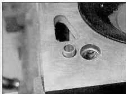
9.46a The locating dowel in the cylinder block
