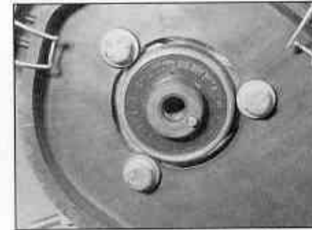
9.31a Bolts securing the inner timing cover to the cylinder head
