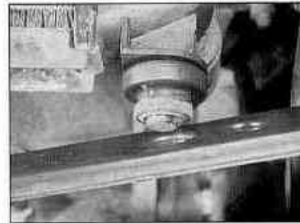
4.57b Removing the bracket from the rubbers on the bottom of the radiator
