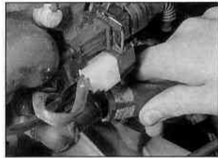
4.45a Disconnecting the heater return hose ...
