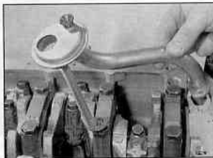
13.4a Removing the oil pump pick-up tube ...
