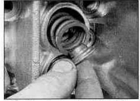
6.16a Removing the upper spring seat ...
