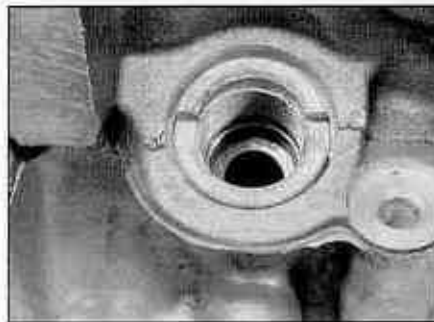
6.18 Swirl chamber retaining collar (diesel engine)
