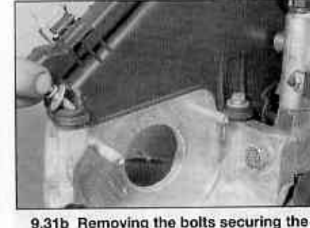
9.31b Removing the bolts securing the inner timing cover to the injection pump/oil filter bracket
