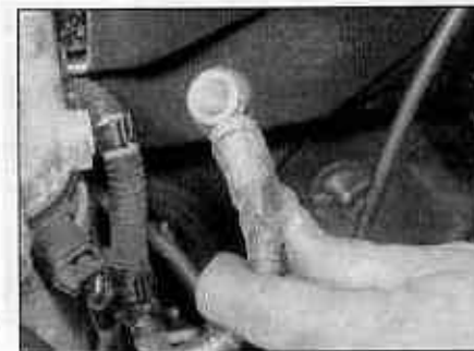
4.42b Cover the end of the hose to prevent dust entry
