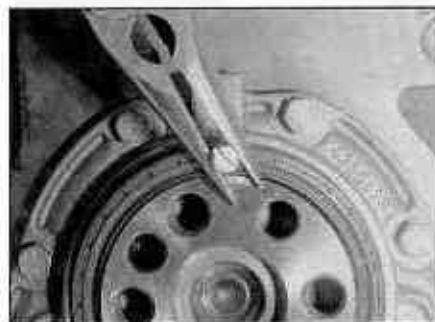
8.8b Using a self-tapping screw and pliers to remove the rear oil seal
