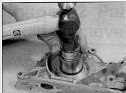
13.14 Fitting the new oil seal to the oil pump casing
