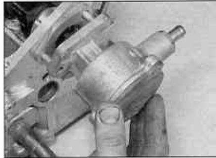
6.8e Removing the vacuum pump
