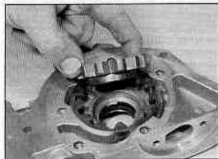
13.8a Removing the inner rotor ...
