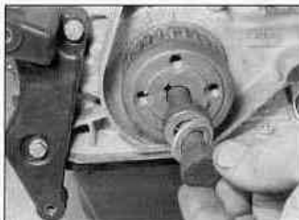
5.22a Unscrew and remove the bolt, washer and spacer ...
