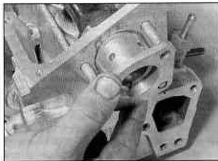
6.9a Removing the camshaft left-hand side mount ...
