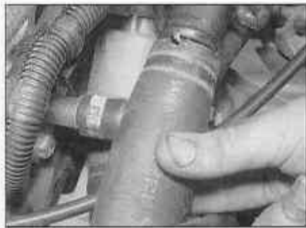
4.44a Disconnecting the radiator top hose from the thermostat housing
