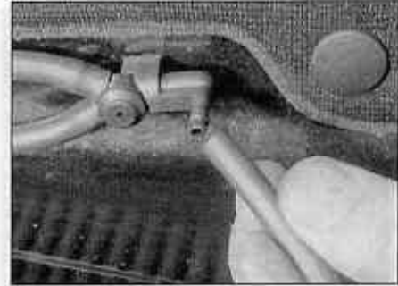
4.1b Disconnecting the washer tubing
