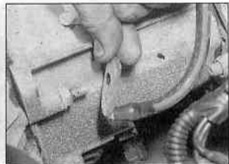
4.8 Disconnecting the earth lead from the transmission
