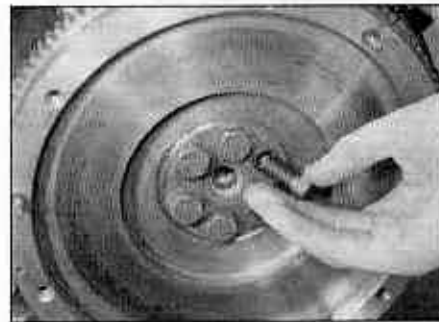
10.8b Inserting the flywheel bolts
