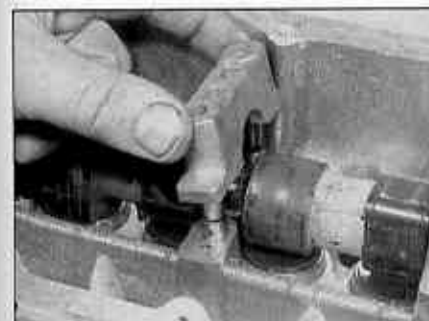
6.12b ... and remove the bearing caps
