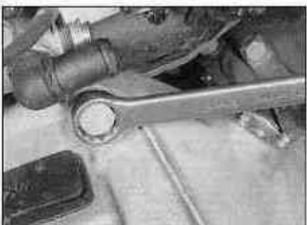
4.82a Unscrewing the transmission-to-engine bolts
