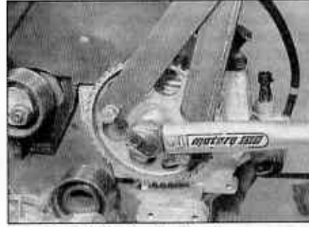
5.35 Tightening the injection pump sprocket bolt
