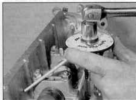
9.53 Angle-tightening the cylinder head bolts to the Stage 3 and Stage 4 settings
