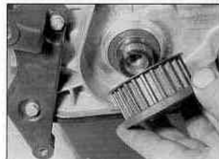
5.22b ... and remove the crankshaft sprocket
