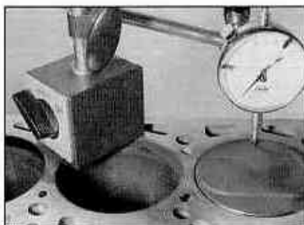
9.42 Checking the piston protrusion with a dial gauge
