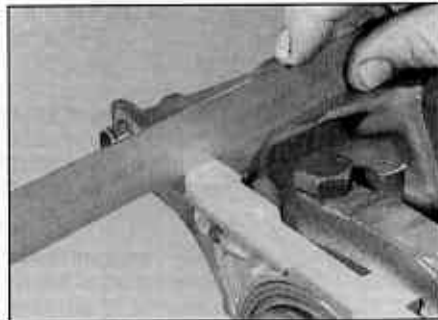
13.19 Checking that the oil pump and sump mating surfaces are correctly aligned with a straight-edge
