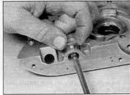
13.9a Depress the relief valve collar and remove the retaining plate ...
