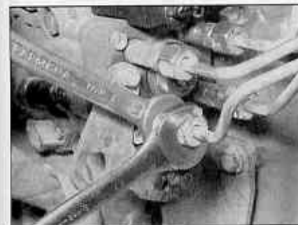
9.24 Unscrewing the union nuts from the injection pump
