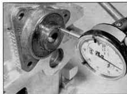
6.32 Checking the camshaft endfloat with a dial gauge
