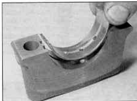
12.8 Locating a lower half main bearing shell in its cap
