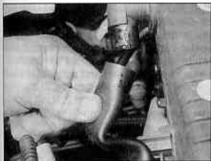
2.4a Disconnect the large breather hose ...
