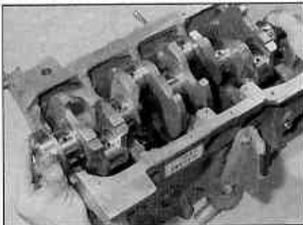
12.5 Lowering the crankshaft into the crankcase
