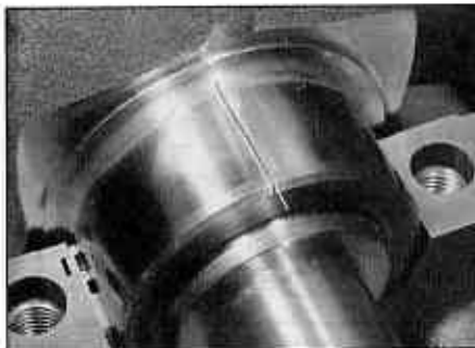
12.7 Lay the Plastigauge on the main bearing journals
