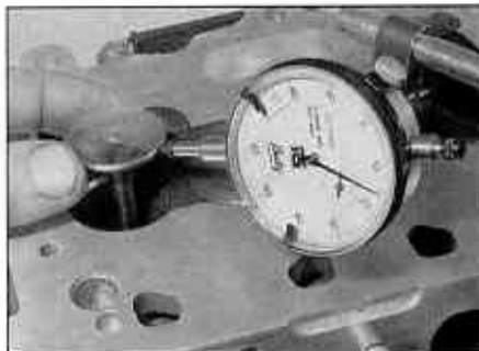
6.27 Checking the valve guides and valves for wear
