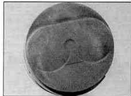
7.26c Piston crown on diesel engines
