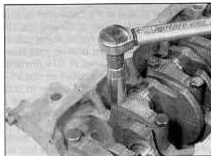
12.10b . . . and torque-tighten them
