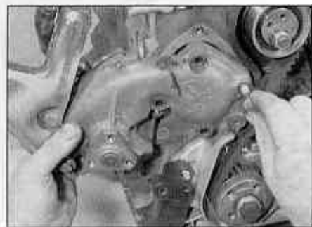
7.11 Removing the coolant pump assembly (diesel engine)
