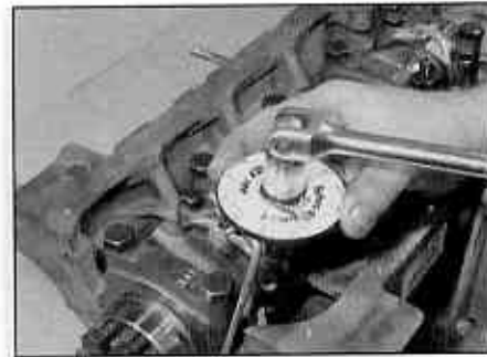
7.43b Angle-tightening the big-end bearing cap bolts (diesel engine)
