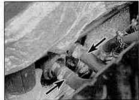
8.3 Slacken the clips (arrowed) and detach the heater unit coolant hoses from the ports at the bulkhead
