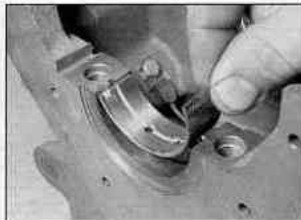
8.8b . . . and upper bearing shells (diesel engine)
