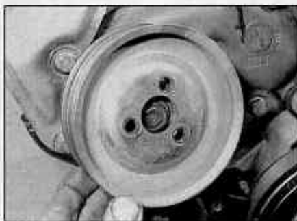
7.9b . . . and lift off the pulley (diesel engine)
