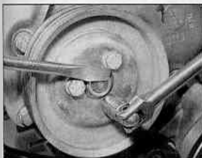
7.9a Unscrew the coolant pump pulley bolts . . .
