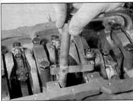
9.1a Removing the oil return tube from the crankcase
