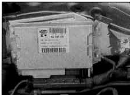
5.40 ECU located on the right-hand inner wing
