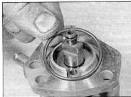
6.55a Fitting a new large O-ring on the vacuum pump
