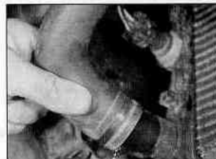
3.4a Slacken the clip and disconnect the radiator bottom hose
