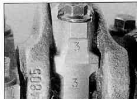
7.8b Connecting rod and cap numbers (petrol engine)
