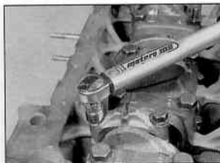
7.43a Torque-tightening the big-end bearing cap bolts (diesel engine)
