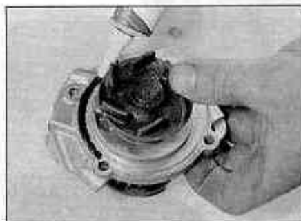
7.17 On petrol engine models, apply a continuous bead of sealant (liquid gasket) to the pump mating face
