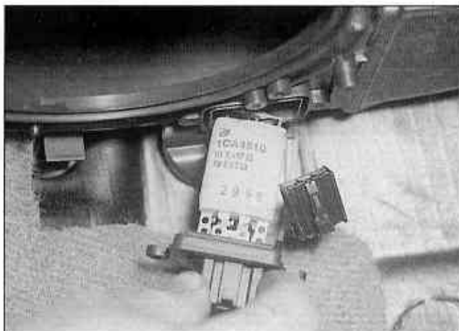
8.21b . . . and withdraw the resistor from the blower unit case
