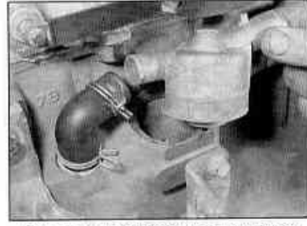
9.1e Removing the oil vapour breather casing
