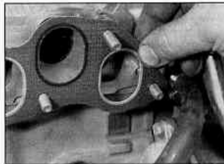
5.14 Removing the exhaust manifold gasket (diesel engine)
