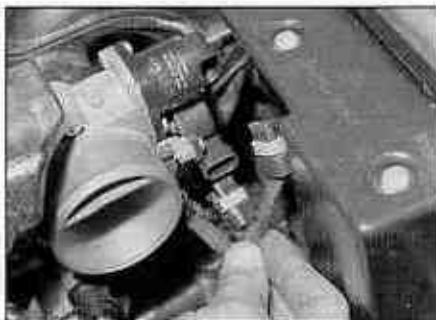
6.3 Disconnect the wiring connectors from the throttle potentiometer and the idle control stepper motor
