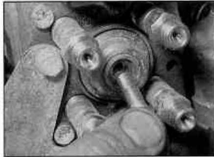
7.4 Unscrew the access screw from the rear of the injection pump (Bosch)
