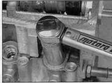
9.13 Tightening an injector with a torque wrench
