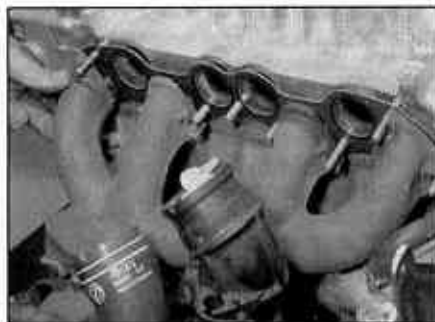
5.12 Removing the exhaust manifold (diesel engine)
