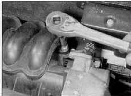
6.14a Undo the inlet manifold upper section retaining bolts ...
