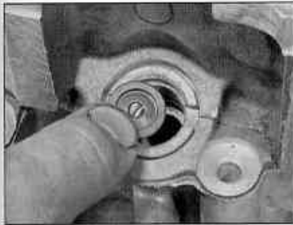
9.9 Removing the fire seal washer
