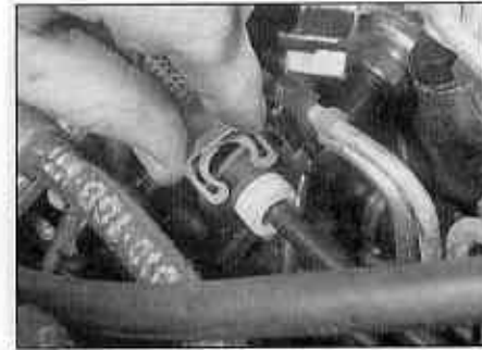
3.8 Removing the spring clip from the accelerator outer cable
