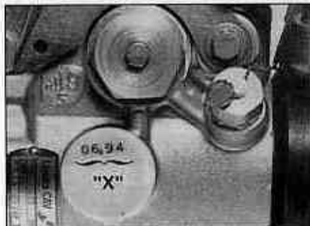
8.7a Pump timing value (x) marked on plastic disc (Lucas)
