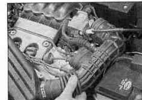
2.12 Removing the air cleaner and inlet air duct assembly
