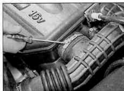
2.7 Release the hose clip and disconnect the inlet air duct from the resonator
