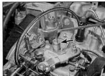
8.4 Removing the injection pump timing inspection plug (Lucas)
