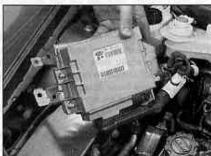
6.35 Undo the mounting bracket nuts and withdraw the ECU from the inner wing
