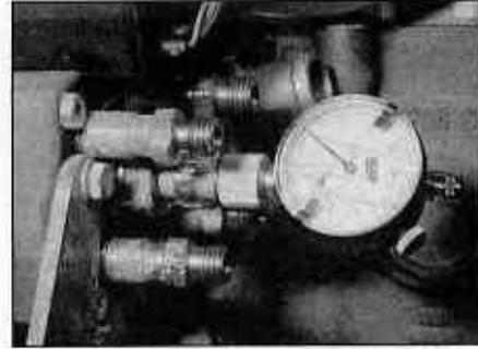
7.5 Dial gauge and adapter (Bosch)
