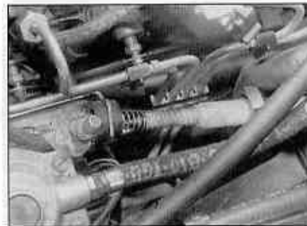
3.3 Removing the outer cable
