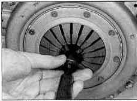
7.17 Using a clutch friction plate centralising tool
