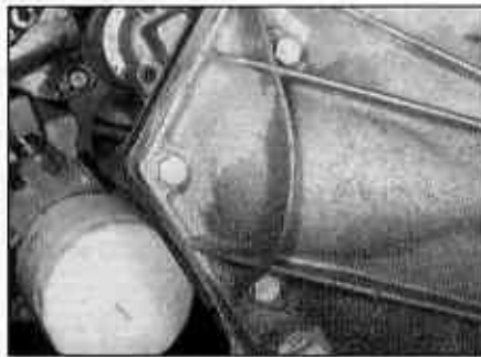
8.6a Starter motor mounting bolt locations (diesel engine)
