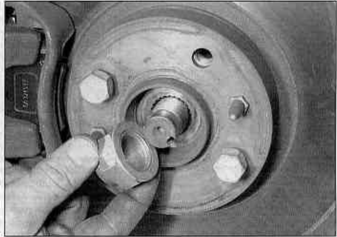
2.13 Fitting a new driveshaft nut
