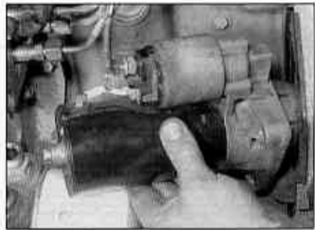
8.6b Removing the starter motor (diesel engine)
