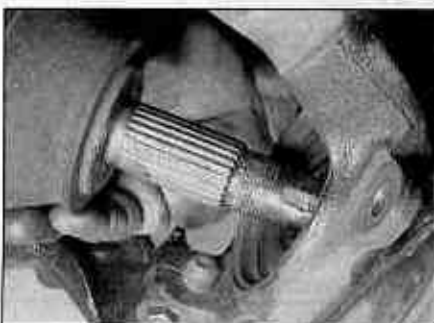
2.5 Extracting the driveshaft from the hub carrier
