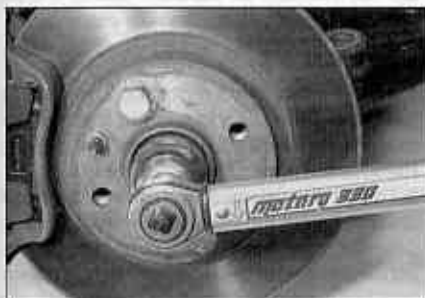
2.20a Tighten the driveshaft nut to the specified torque (roadwheel removed for clarity)
