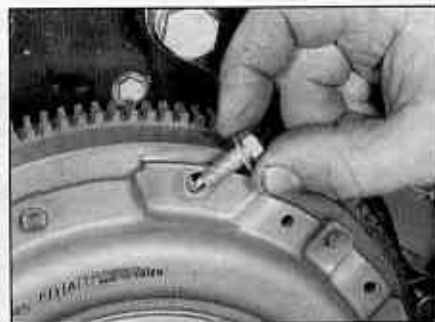
7.3 Removing the clutch pressure plate bolts
