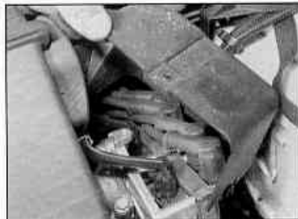
3.1 Removing the ignition coil cover
