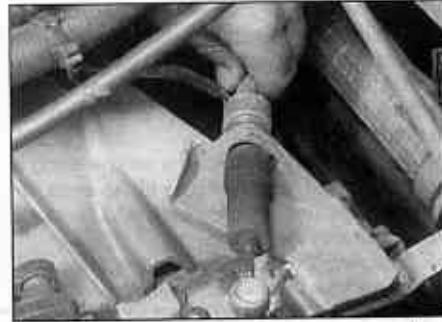
3.9b Removing the gear engagement cable from the mounting bracket
