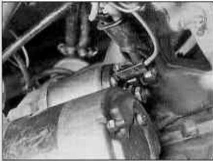
8.4a Starter motor wiring connections (petrol engine)
