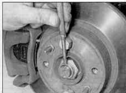
2.20b Stake the rim of the nut into the recess in the driveshaft
