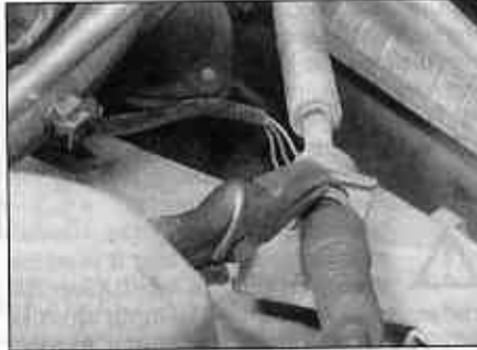
3.9a Remove the clip to release the gear engagement cable
