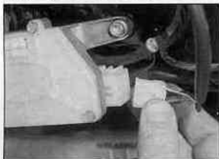
15.4a Working inside the tailgate, unplug the tailgate wiper motor wiring at the connector ...
