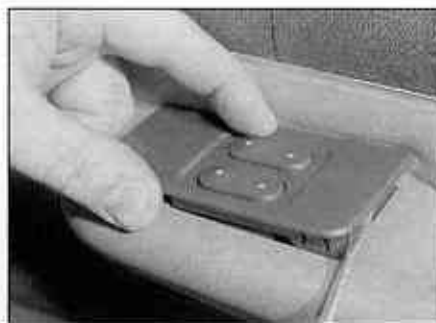
14.4a Prise the electric window/mirror adjustment switch from the armrest ...
