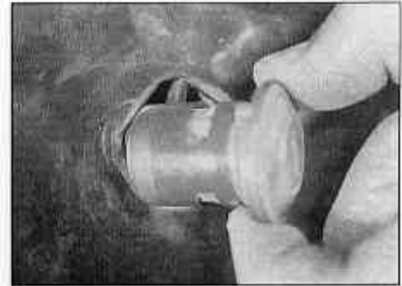
16.7b Extract the lock cylinder from the door
