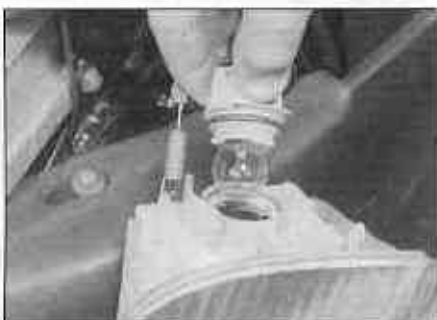
4.23 Twist the bulbholder anti-clockwise and withdraw it from the light unit
