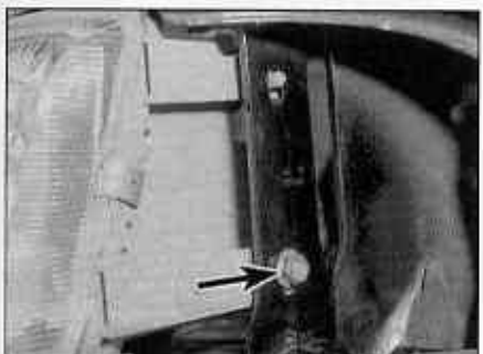
6.3a Unscrew the headlight side securing bolt (arrowed) . . .
