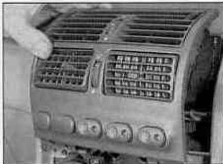
19.8 Remove the combined ventilation/switch panel from the facia
