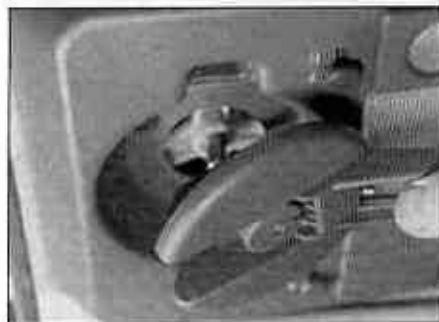
5.3a On models with a manually operated sunroof, remove the sunroof crank handle
