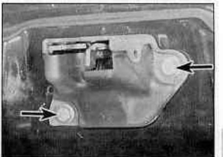
10.1 Unscrew the bolts (arrowed) securing the lock assembly to the lower edge of the tailgate
