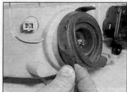
4.4 Pull the rubber boot from the rear of the headlight unit
