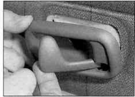
14.3b ... then prise out the door grab handle moulding
