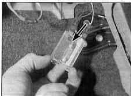
5.10 The bulb can be prised from its spring-loaded contacts (arrowed)
