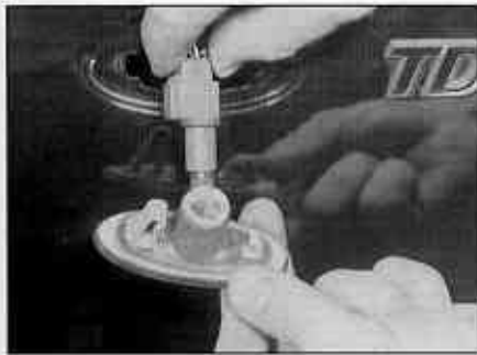
4.27 Withdraw the light unit, then twist the bulbholder anti-clockwise to release it from the light unit
