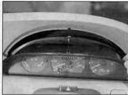
7.3a Carefully pull the panel away from the fascia
