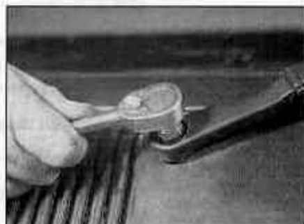
18.3b ... then slacken and remove the spindle nut
