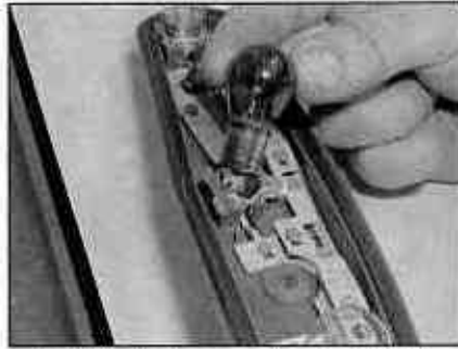
4.40 The bulbs are a bayonet fit in the bulbholder
