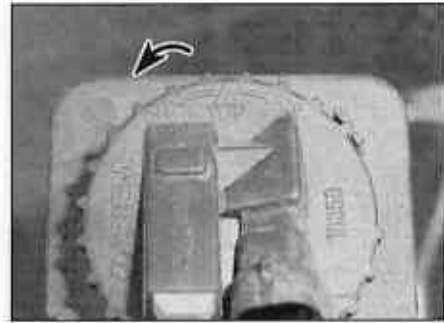
4.33 Unscrew the rear cover from the foglight unit by turning it anticlockwise
