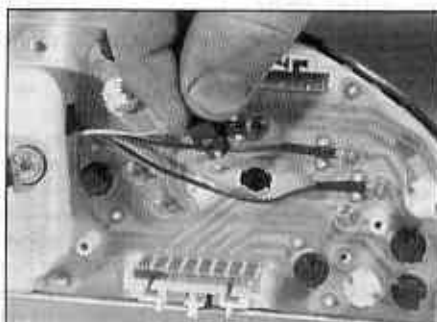
5.13 The bulbs are a bayonet fit in the rear of the instrument panel
