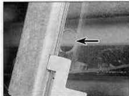
18.4b Disengage the regulator mechanism from the hole (arrowed) at the base of the window glass
