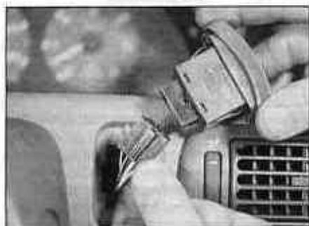
14.10 Unplug the wiring from the rear of the switch body at the connector
