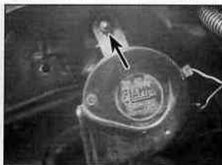
9.3 Unscrew the securing bolt (arrowed) and remove the horn sounder
