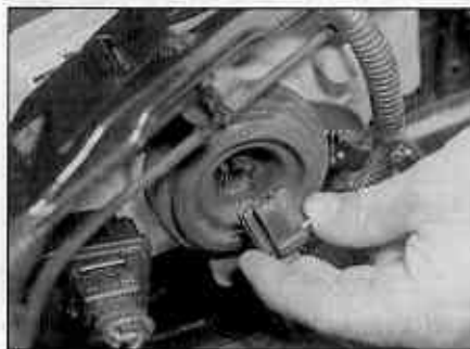
4.3 Pull the wiring plug from the rear of the bulb
