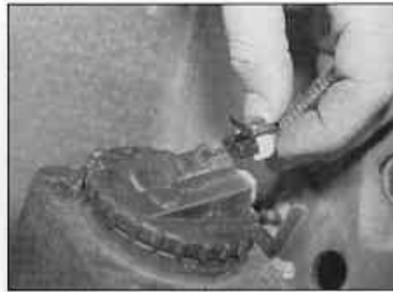
4.32 Disconnect the wiring from the rear of the foglight unit at the connector
