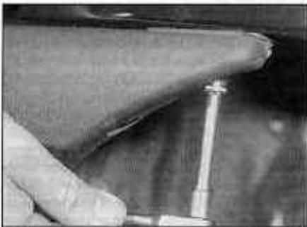
7.3 Remove the retaining screws from the leading edges of the bumper moulding
