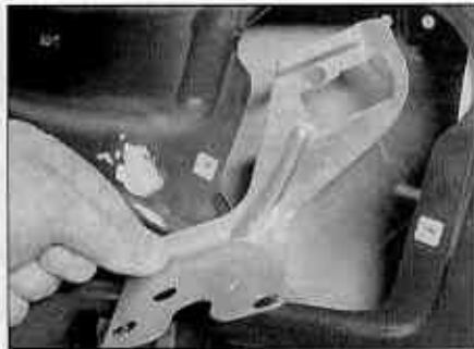
16.3 Unbolt and remove the anti-theft bracket from the rear of the door handle
