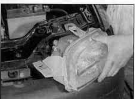
6.4 Withdraw the headlight unit from the vehicle
