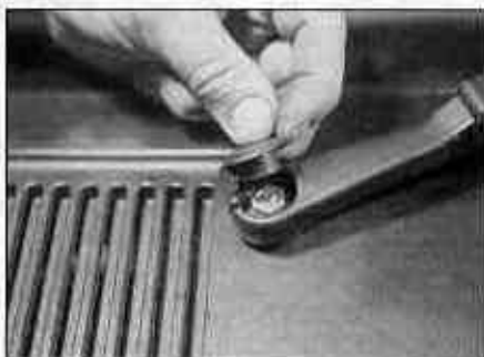
18.3a Lift up the wiper arm spindle nut cover ...
