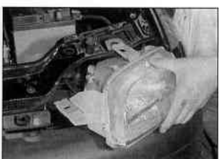
6.6 Disconnecting the direction indicator light unit wiring from the bulb holder
