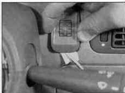
14.9 Carefully lever the switch body out of the fascia, using a flat bladed instrument
