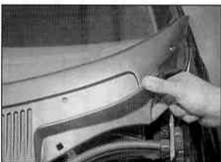
17.3b ... and withdraw the cowl panel
