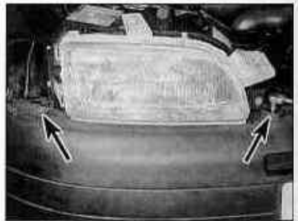
6.6 Remove the retaining bolts (arrowed) from either side of the headlight units
