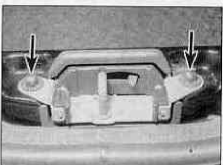
10.6 Slacken and unscrew the bolts (arrowed) securing the striker plate to the bodywork
