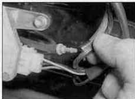
15.4b ... and disconnect the washer hose at the union
