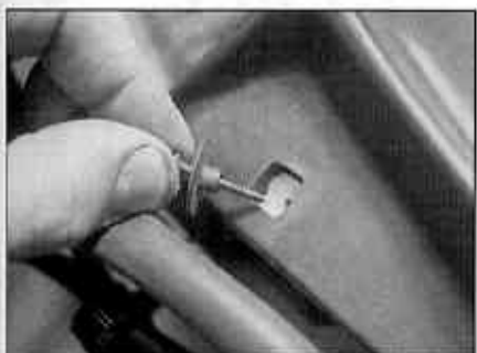
17.3a Remove the securing screws and plastic clips ...
