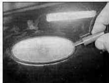
4.26 Slide the light unit towards the front of the vehicle slightly, then insert a plastic implement behind the rear edge
