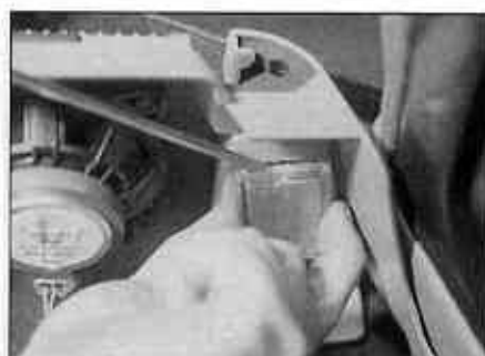
5.9 Unclip the lens from the support panel
