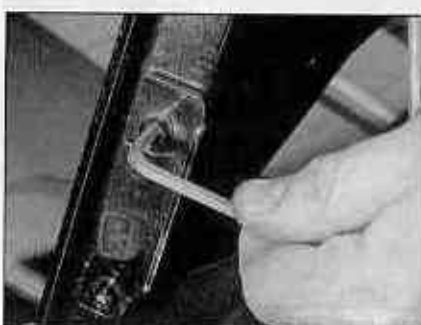
11.3 Slacken and unscrew the bonnet hinge bolts
