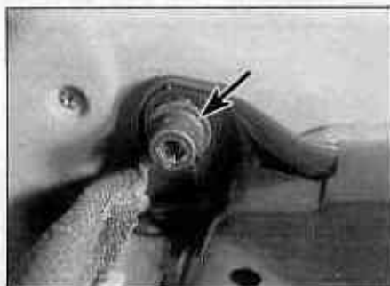
20.8 Remove the bolt (arrowed) and detach the backrest from the mounting bracket
