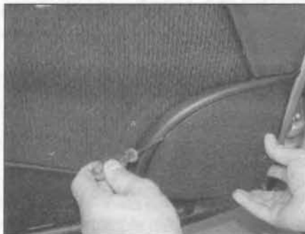
14.5a Prise off the loudspeaker grille ...
