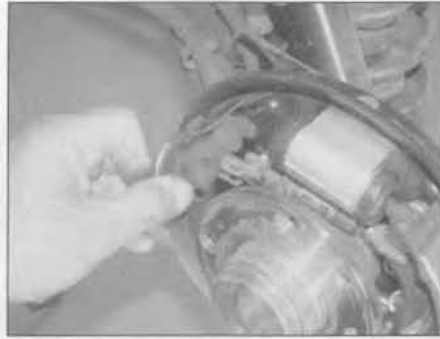
8.8a Remove the leading brake shoe from the backplate . . .
