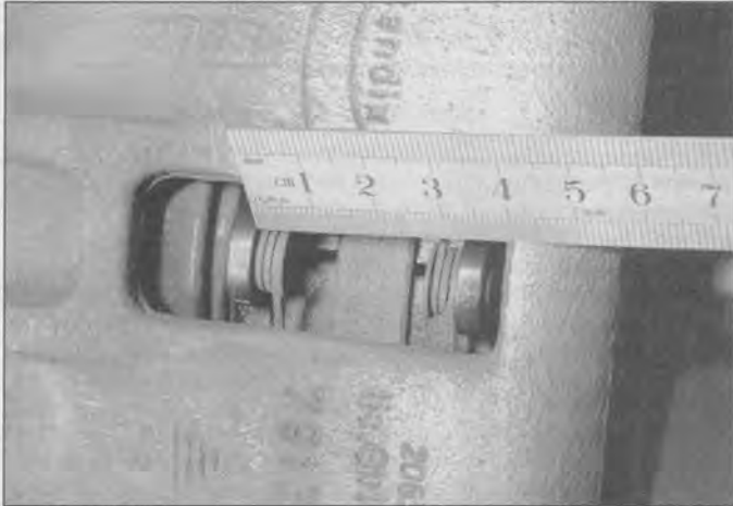
6.2 Check the thickness of the pad friction material through the hole on the front of the caliper
