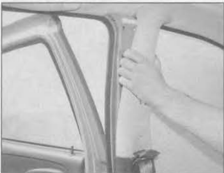
25.26 Carefully pull the panel away from the pillar to release the securing clips – 5-door models
