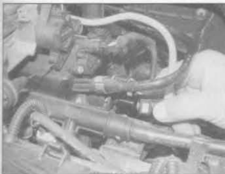
11.7b . . . and fuel vapour hose from the evaporative emission control solenoid – SOHC (8-valve) engines
