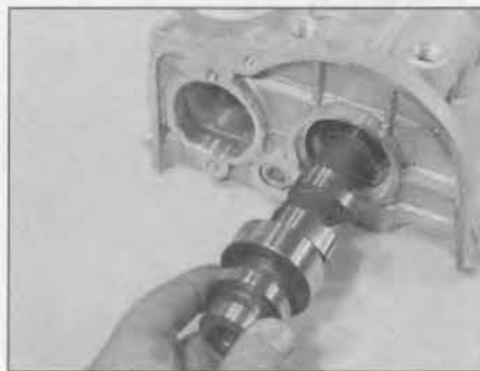
10.11 . . . then remove the exhaust camshaft from the cylinder head extension
