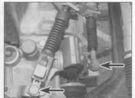
4.9 Disconnect the selector cable end fittings (arrowed) from the transmission lever ball-studs – manual transmission models
