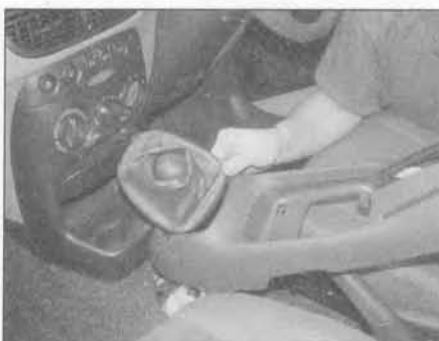
26.11 Feed the gear lever boot through the aperture and remove the console – manual transmission models
