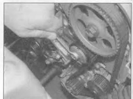
5.16 Release the nut on the timing belt tensioner ...
