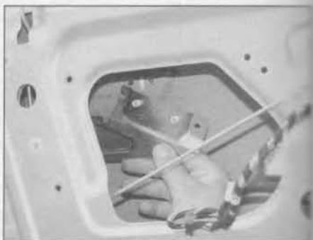
16.4 Unbolt and remove the lock shield from the rear of the door handle
