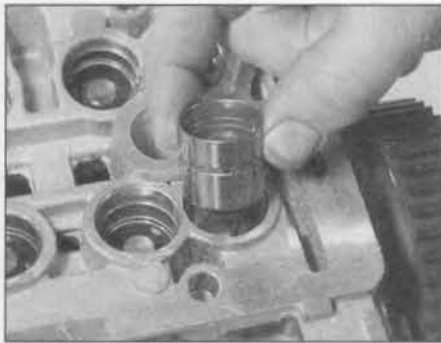
10.3 Remove the cam followers from their locations in the cylinder head extension
