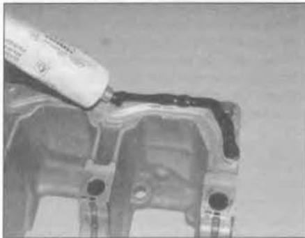
17.13 Apply a 2.0 mm bead of silicone sealant to the lower crankcase mating surface – DOHC (16-valve) engines
