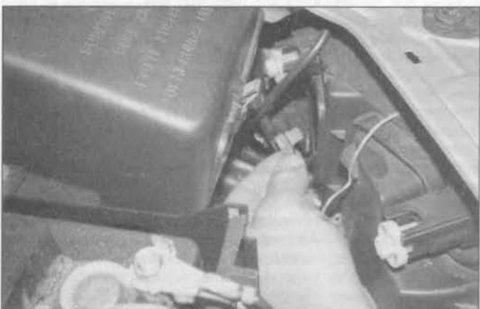
4.4 Disconnect the wiring connector from the rear of the dipped beam bulb
