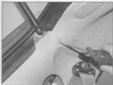
25.51a Undo the screws securing the upper section of the parcel shelf support to the inner wing . . .
