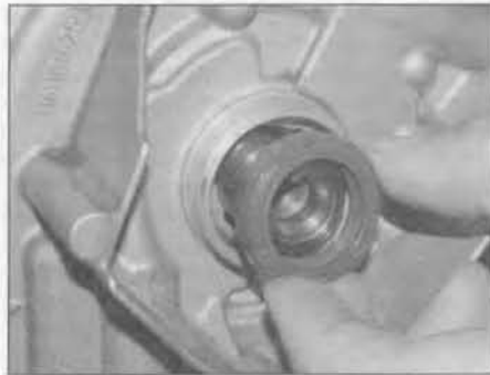
9.4 Locate the new oil seal on the oil pump casing with the sealing lips facing inwards
