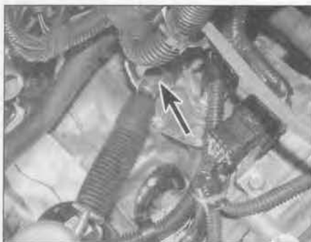
2.4 Undo the nut (arrowed) and withdraw the selector cable from the support bracket
