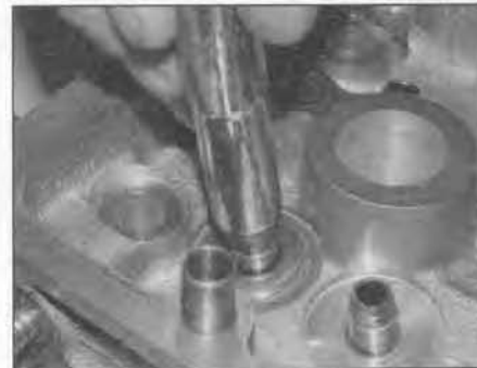
8.2 Use a suitable socket or metal tube to press the valve stem oil seal firmly onto the guide
