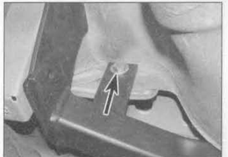
28.15b . . . and attach the upper mountings (arrowed) with the bolts, nuts, flat washers and lockwashers
