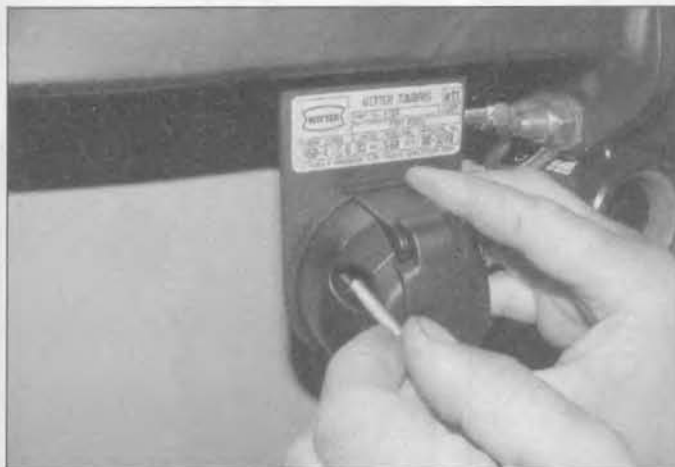
21.8a Locate the electrical socket on the mounting plate and insert the retaining screws . . .
