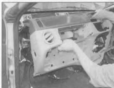
27.40 Carefully pull the facia moulding away from the bulkhead
