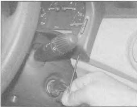
27.10 Undo the two instrument panel surround lower retaining screws
