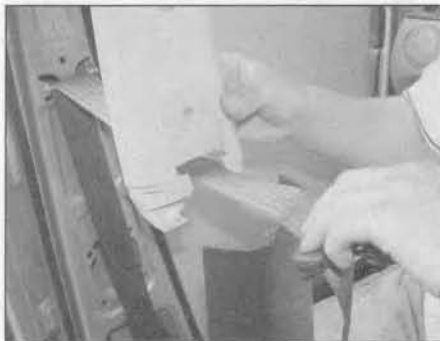
25.27 Separate the upper section of the panel from the lower section and disengage the seat belt – 5-door models
