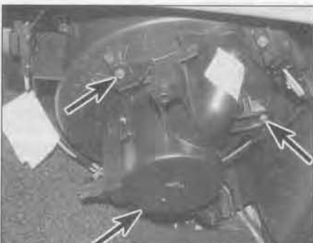
8.17 Undo the three screws (arrowed) securing the blower motor to the underside of the heater assembly
