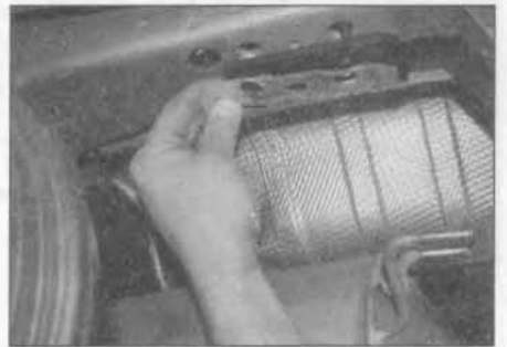
28.13b . . . followed by the previously removed exhaust heat shield . . .
