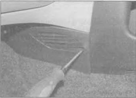
27.14a Undo the retaining screws securing the vent panels to the lower centre panel . . .
