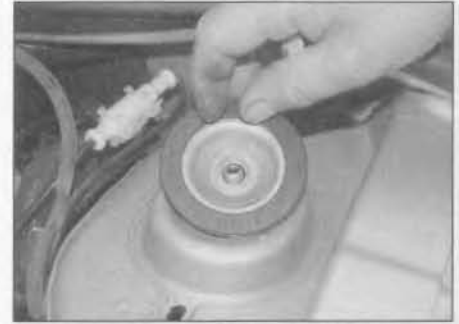
4.5b . . . lift off the mounting cup and withdraw the strut from under the wheel arch
