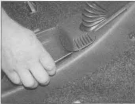
26.15 Carefully prise up and remove the coin holder from the console – automatic transmission models
