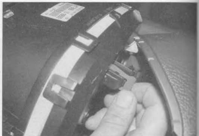
7.5 Lift up the wiring connector locking catch and disconnect the connector
