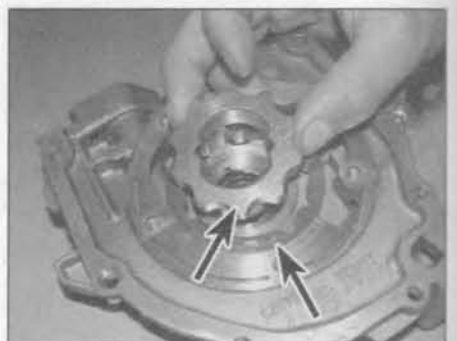
15.10 After inspection, refit the pump rotors with the orientation marks (arrowed) facing upwards
