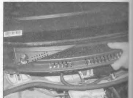
22.5 . . . then lift the panel up at the front and move it forward to disengage the rear clips
