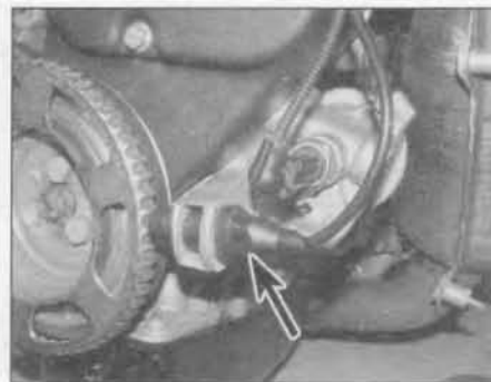
9.26 Crankshaft TDC sensor location (arrowed)
