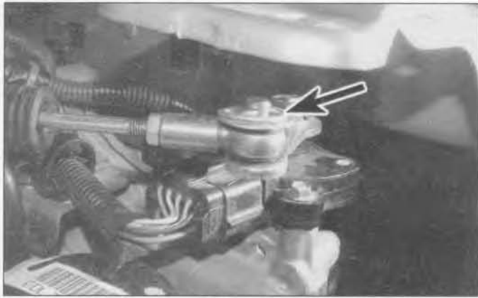
2.3a Extract the selector cable end fitting retaining clip (arrowed) . . .
