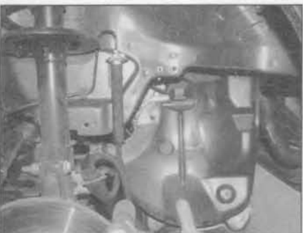
4.12 Undo the retaining screws and remove the wheel arch liner main and centre panels
