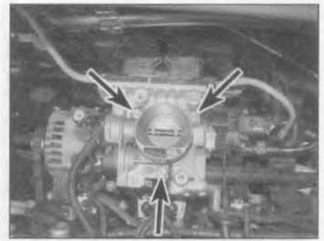
9.7 Throttle body retaining bolts (arrowed)
