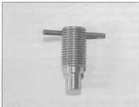
2.6a To make an alternative camshaft locking tool ...
