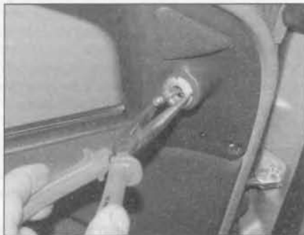
10.3b Using pointed-nose pliers, unscrew and remove the locking collar
