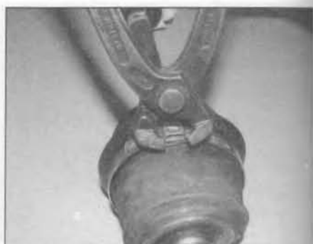
3.15 Locate the large securing clip over the gaiter and secure the clip by compressing the raised portion
