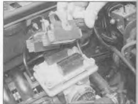
10.44 Rotate the locking catches and disconnect the two wiring connectors from the top of the ECU
