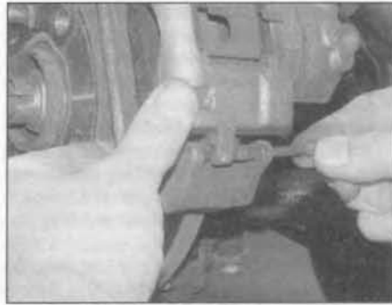
4.3b . . . and extract the lower guide pin from the caliper – SOHC (8-valve) engine models
