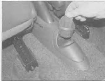
12.8 lift out the ashtray from the rear of the centre console
