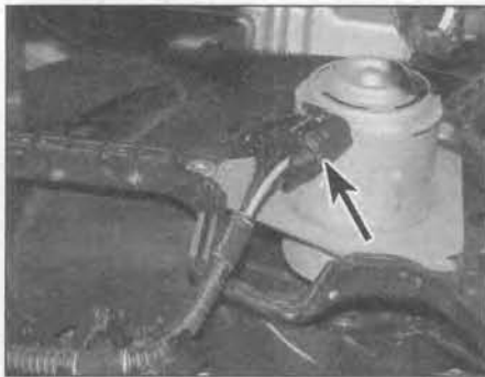
5.8 Disconnect the wiring connector (arrowed) from the electric fan motor
