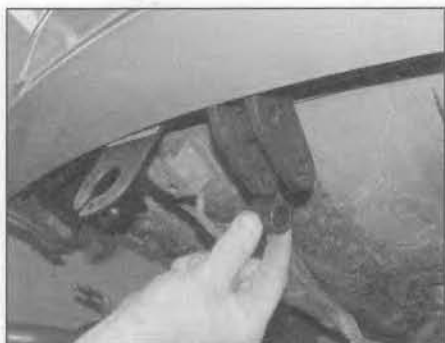
28.17a If the fixed towball is to be used, locate the two spacing bushes between the mounting flanges in the cross-bar
