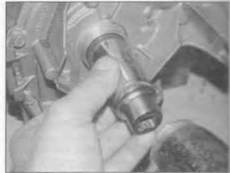
9.5 Using a suitable tubular drift, drive the oil seal squarely into the casing
