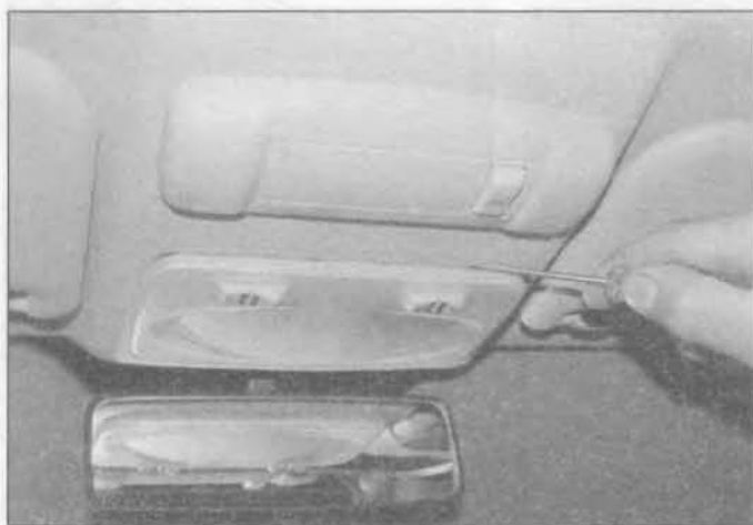
5.2 Carefully prise the courtesy light unit from its location
