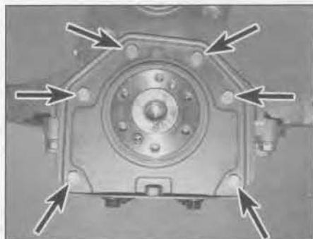
8.9 Undo the retaining bolts (arrowed) and remove the crankshaft left-hand oil seal housing complete with integral oil seal
