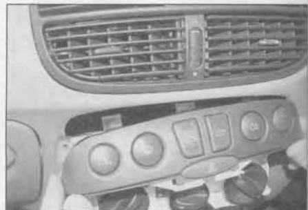
27.21 Lower the panel to free the upper retaining tags, then disconnect the wiring connectors
