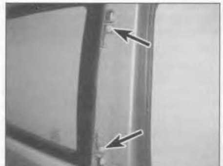
19.3 Undo the hinge retaining bolts (arrowed) and withdraw the glass from the window aperture
