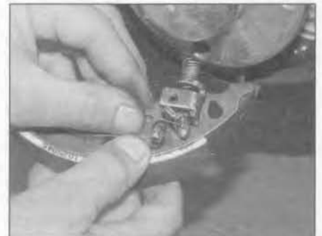
8.10 Lift the locking catch on the trailing shoe handbrake lever, and slide out the handbrake cable end
