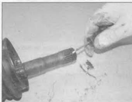
3.4 Remove the circlip from the groove in the driveshaft splines
