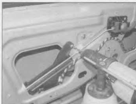
16.3 Drill out the pop rivets securing the anti-theft partition to the front door panel
