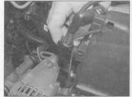
4.8 Disconnect and release the wiring harness from the upper timing cover
