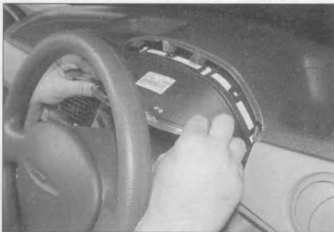
7.4 Tip the panel down at the top and pull the it away from the fascia slightly
