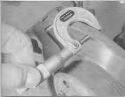
6.8 Measuring brake disc thickness with a micrometer
