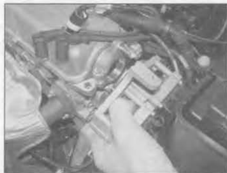
2.18b . . . and remove the ignition coils, complete with mounting bracket
