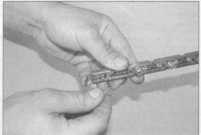
4.43 Remove the relevant push-fit bulb from the bulbholder
