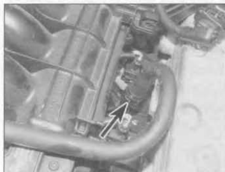
10.10 Fuel supply pipe quick-release connector (arrowed)
