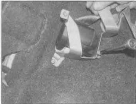
24.24 Undo the bolts and remove the audio amplifier/loudspeaker unit mounting bracket – 5-door models
