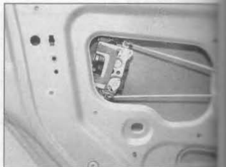
16.45 Manoeuvre the lock mechanism and link rods out through the door aperture
