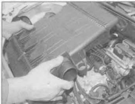
2.10b . . . then lift the air cleaner casing off the engine
