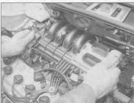
11.31b . . . and remove the inlet manifold from the cylinder head – DOHC (16-valve) engines
