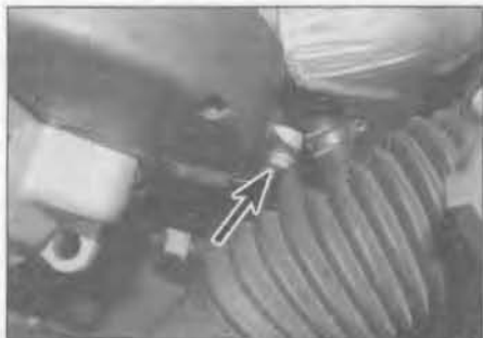
4.3b ... and the front retaining bolt (arrowed) located behind the air cleaner intake duct
