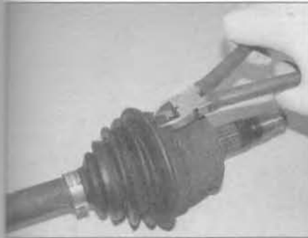
3.2 Release the rubber garter retaining clips by cutting them off with side-cutters
