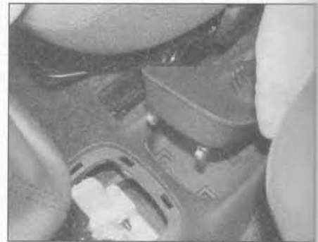
26.3 Carefully prise up the front of the oddments tray to release the two retaining clips – manual transmission models
