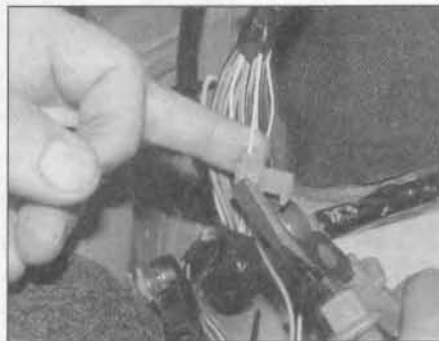
21.24 Connect the towbar socket and audible warning unit wiring to the vehicle harness using snap connectors
