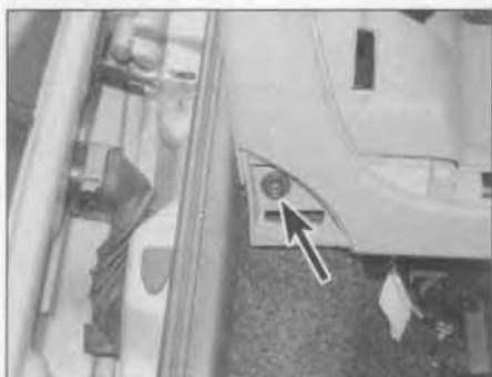
27.39d ... and the lower bolt (arrowed) on each side
