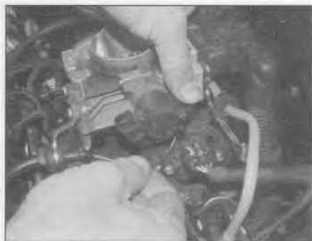
3.2a Disengage the accelerator inner cable from the throttle cam . . .
