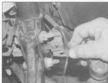
2.7a On models with ABS, release the wheel speed sensor cable from the suspension strut brackets . . .
