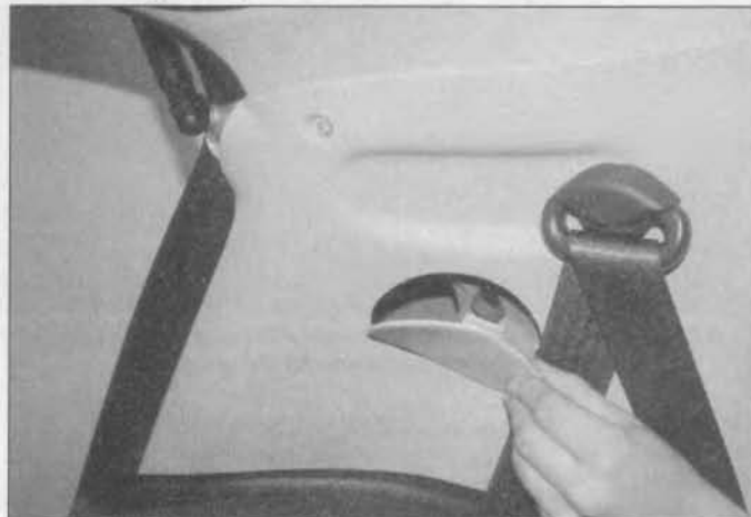
4.29 Prise the plastic cap from the rear pillar trim panel
