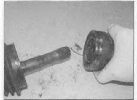
3.3b . . . then withdraw the outer joint from the driveshaft
