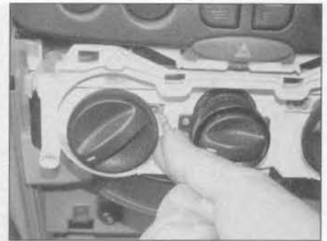
5.13 Remove the relevant push-fit bulb from the heater/ventilation control panel
