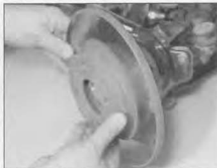
6.18b . . . and lift the disc off the wheel hub
