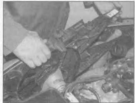
5.10c ... then lift out the cooling fan assembly
