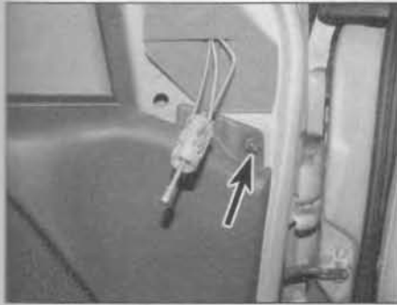
14.9 Undo the screw (arrowed) at the upper front corner of the panel, and the remaining screws securing the lower edge
