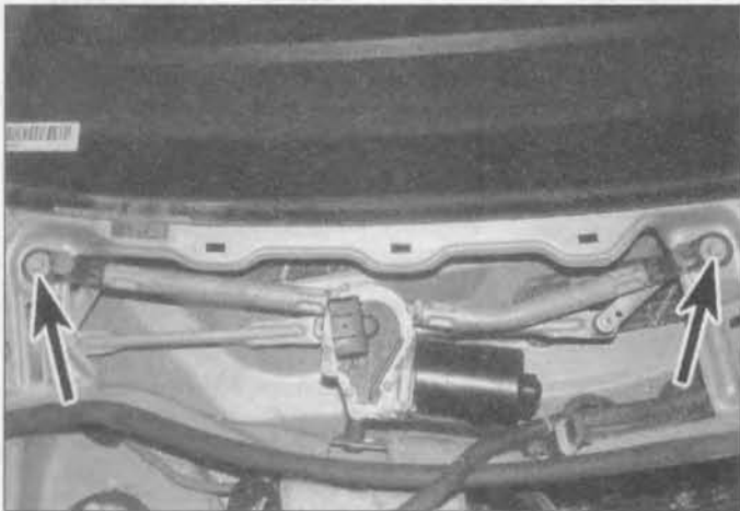
16.5a Undo the two wiper motor and linkage retaining bolts (arrowed) . . .
