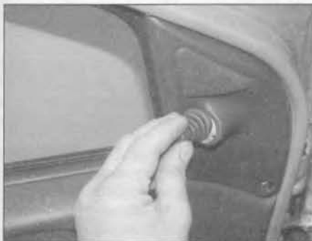
10.3a On manually-adjustable mirrors, prise the rubber cover off the adjustment lever
