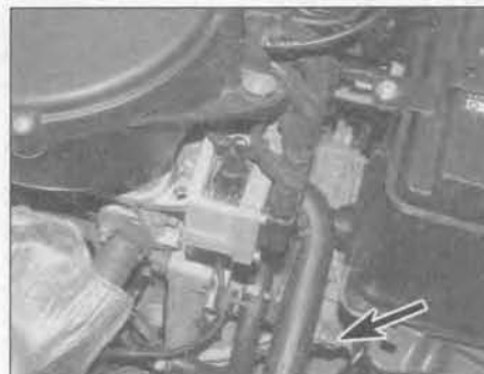
24.2 Manual transmission oil filler/level plug location (arrowed)
