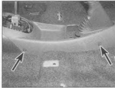
26.16 Undo the two screws (arrowed) on each side of the console – automatic transmission models
