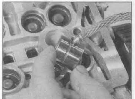
10.24 Lubricate the cam followers and place them in position in their respective bores
