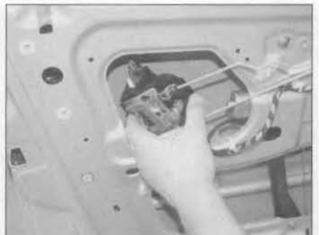
16.26 Manoeuvre the lock mechanism and locking knob link rod out through the door aperture
