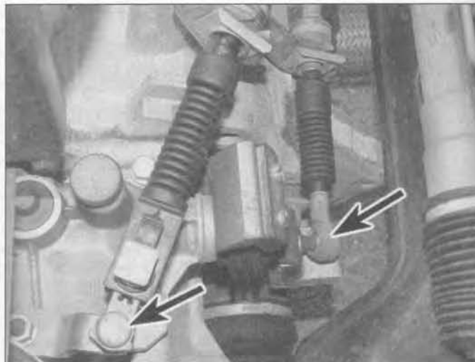
3.2 Disconnect the selector cable end fittings (arrowed) from the transmission selector levers
