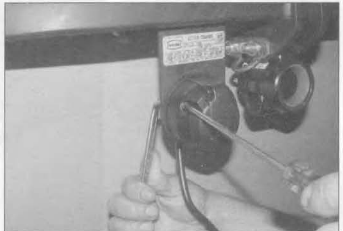
21.8b . . . then secure the screws with the retaining nuts
