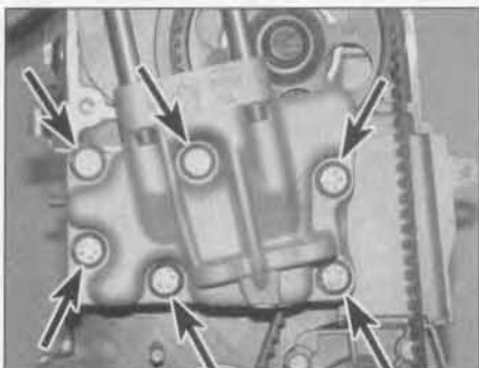
5.9a Undo the six bolts (arrowed) . . .
