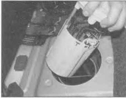
6.8a Lift the fuel pump and sender unit assembly out of the fuel tank . . .
