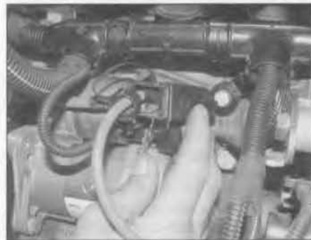
8.5 Raise the plastic cover over the starter solenoid wiring terminals
