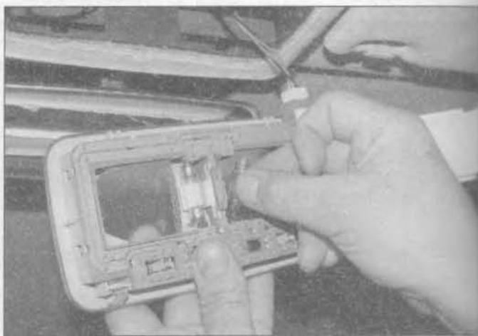
5.4 Remove the relevant festoon bulb from the bulbholder contacts
