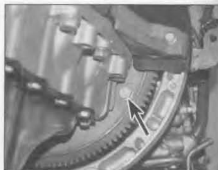
6.22 Torque converter retaining bolt (arrowed) accessible through the bellhousing opening
