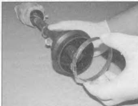
3.11c . . . and the large securing clip
