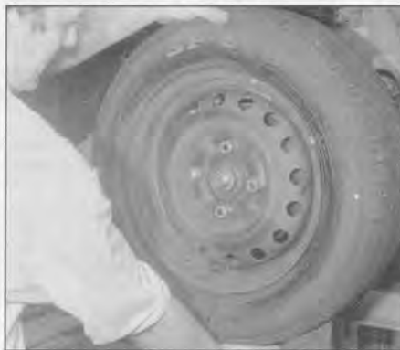
8.3 Rocking a roadwheel to check for wear in the steering/suspension components
