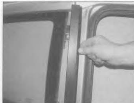
19.2b . . . and lift off the outer trim over the side window hinges
