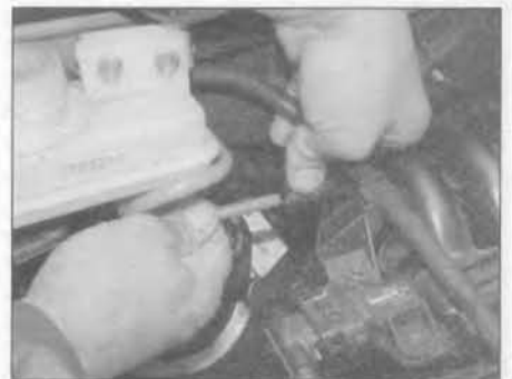
11.21 Disconnect the evaporative emission control vapour hose at the quick-release connector – DOHC (16-valve) engines
