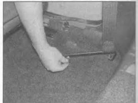
25.32 Undo the bolt securing the front seat belt lower anchor rail to the base of the sill – 3-door models
