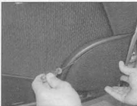
10.5a Prise off the loudspeaker grille . . .
