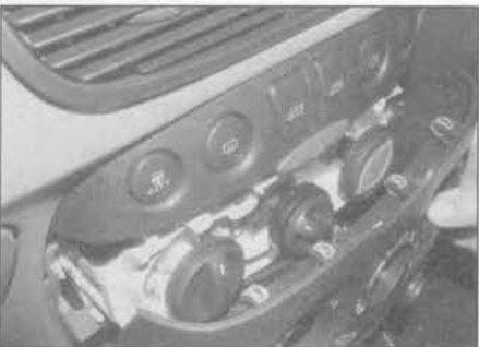
27.16 Carefully prise free the upper edge of the panel to disengage the four retaining clips
