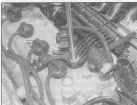
11.29 Undo the bolt securing the inlet manifold support bracket to the cylinder head extension – DOHC (16-valve) engines
