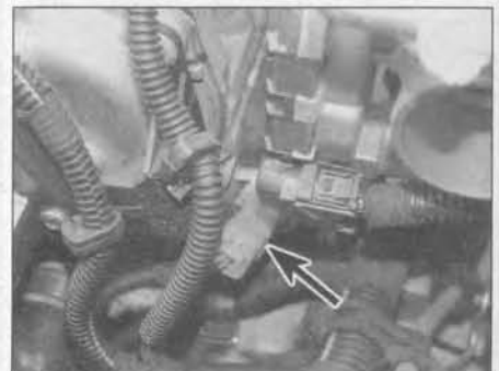
6.1 Engine coolant temperature sensor location (arrowed) on the left-hand end of the inlet manifold
