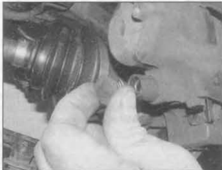
4.7 Prise out the protective covers over the caliper guide pin bolts – DOHC (16-valve) engine models
