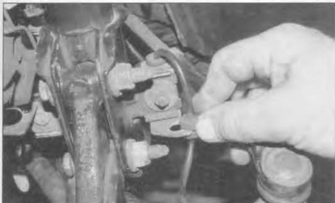
18.17 Unclip the wheel speed sensor wiring from the brackets on the suspension strut
