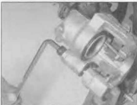
5.5 Unscrew the upper guide pin bolt and remove the caliper from the mounting bracket – SOHC (8-valve) engine models
