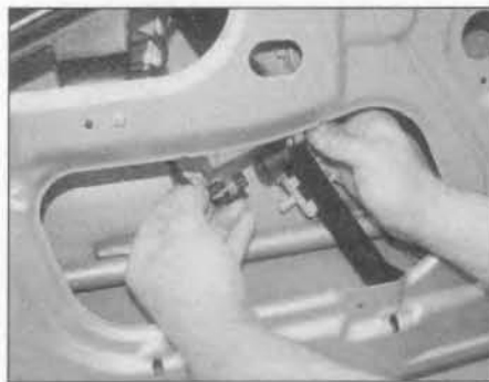
18.15 Lower the regulator assembly and disconnect the motor wiring connector
