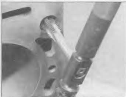
11.8 To clean the cylinder block threads, run a correct-size tap into the holes
