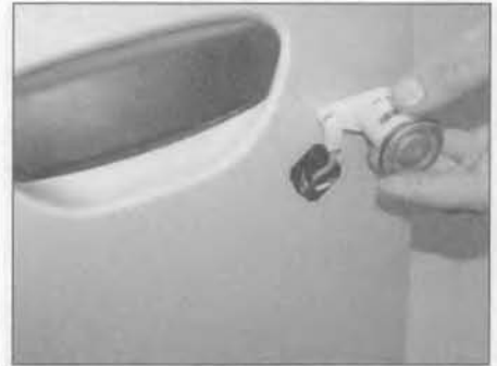
16.12b . . . then remove the cylinder from the door
