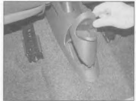
12.9 Undo the retaining screw and remove the ashtray surround
