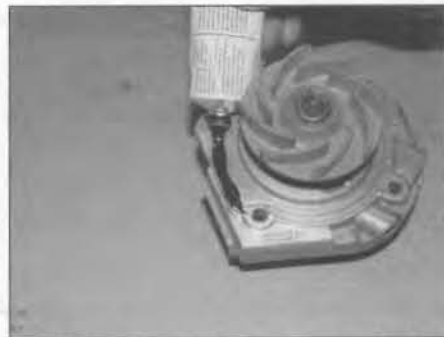
7.7 Apply a continuous bead of RTV sealant to the coolant pump mating face
