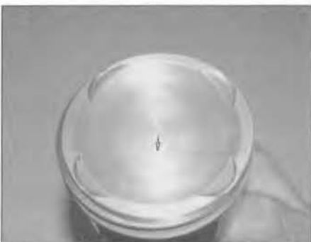
18.8b . . . ensuring that the arrow on the piston crown is pointing towards the timing belt end of the engine
