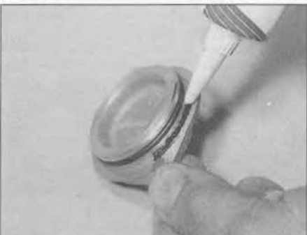
10.22b . . . then apply RTV gasket sealant to the cover plate contact face
