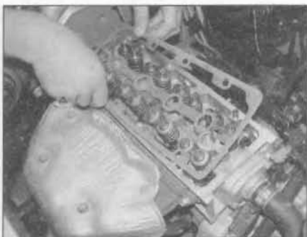
9.8 Locate a new gasket on the cylinder head
