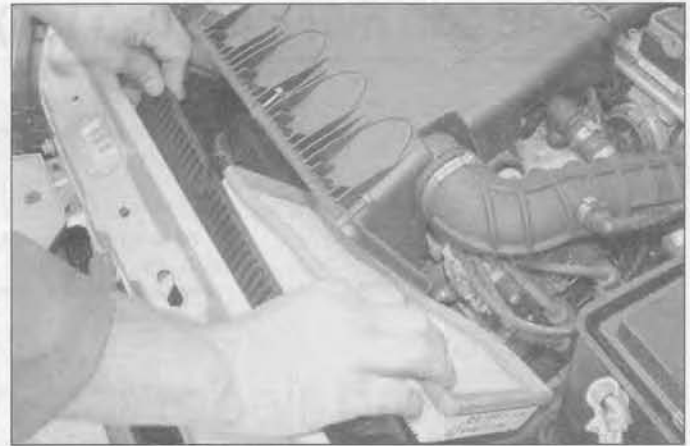
22.5b . . . then tip the cover forward and take out the filter element
