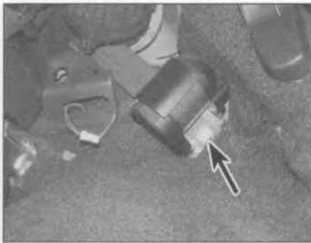
24.17 Rear seat belt inertia reel retaining bolt (arrowed) – 3-door models
