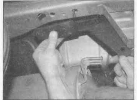
28.13a Locate the left-hand sidearm in position . . .
