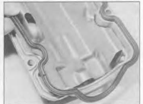
7.10 Ensure that the gasket is correctly seated in the camshaft cover groove
