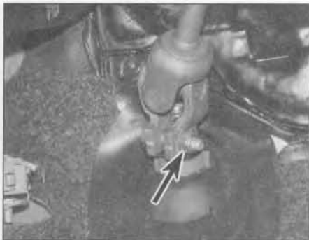
13.6 Unscrew the clamp bolt retaining nut (arrowed) on the intermediate shaft lower universal joint
