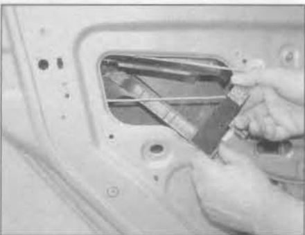
16.40b . . . and remove the window glass lower rear guide channel
