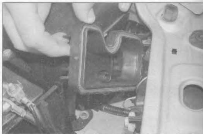
4.3b . . . and lift off the plastic cover from the rear outer corner of the headlight unit
