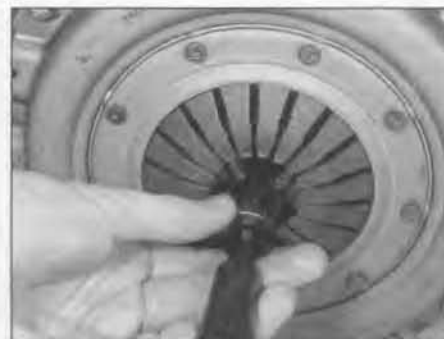
5.16 Using a clutch friction plate centralising tool
