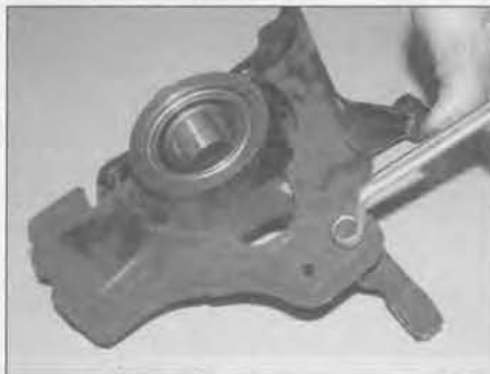
3.4a Undo the retaining bolt . . .
