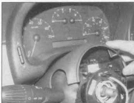
27.8b ... then manipulate the shroud out from under the instrument panel
