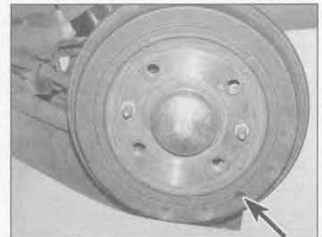
25.2 Check the thickness of the shoe friction material through the hole on the edge of the drum (arrowed)
