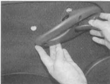
14.4c ... then remove the door interior handle surround
