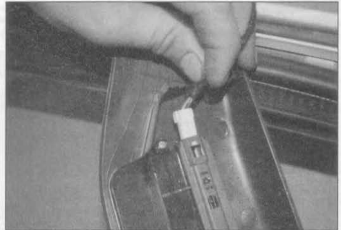
4.41 Withdraw the light unit and disconnect the bulbholder wiring connector
