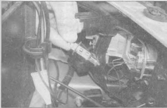
4.10b . . . and remove the bulb from the headlight unit
