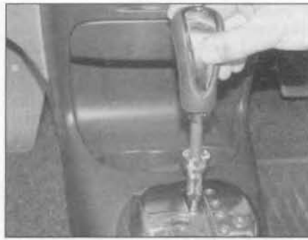
3.2b ... slide the knob off the selector lever ...
