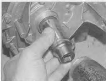
8.5 Using a suitable tubular drift, drive the oil seal squarely into the casing
