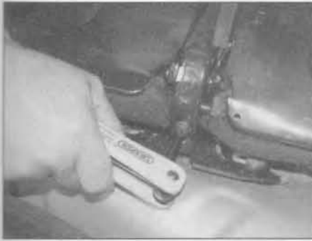
23.7a Undo the retaining bolt and lift up the rear seat back centre hinge locking cover . . .
