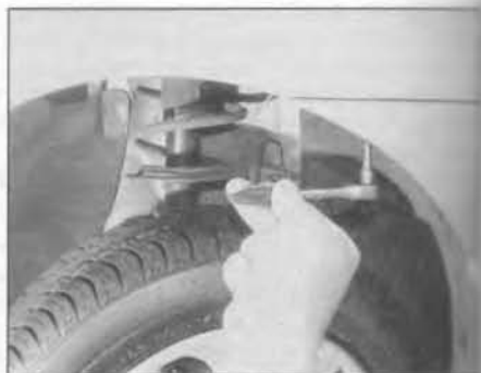
6.3a Undo the two bolts each side securing the upper edge of the bumper to the front wing . . .
