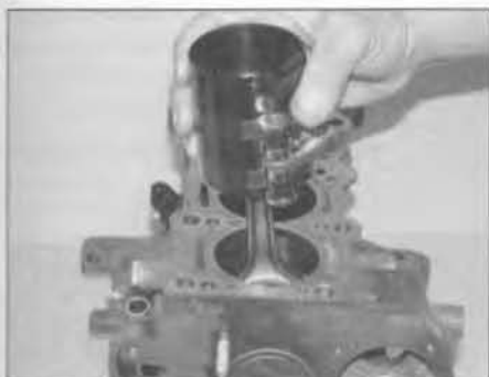
18.8a Insert the piston/connecting rod assembly into the top of cylinder No 1 . . .
