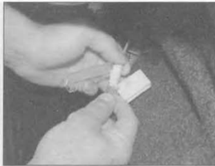
5.8b . . . and remove the push-fit bulb
