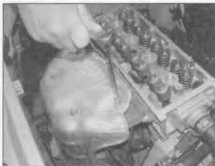
11.2 Undo the upper and lower retaining bolts and remove the exhaust manifold heat shield
