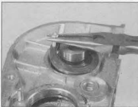
10.10 Extract the exhaust camshaft oil seal . . .
