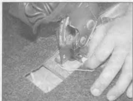
15.2 Disconnect the wiring connector from the handbrake 'on' warning light switch
