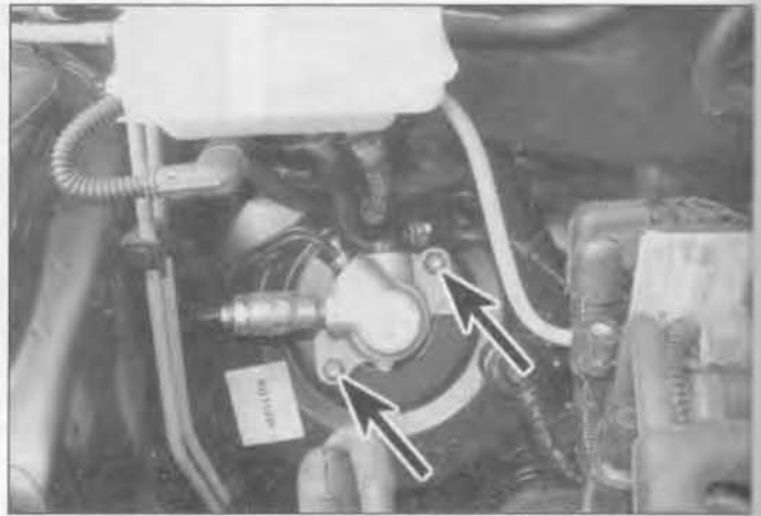
10.5 Master cylinder retaining nuts (arrowed)
