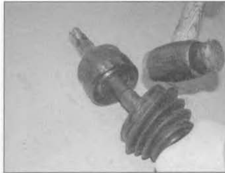
3.3a Sharply strike the edge of the outer CV joint to release it from the internal circlip . . .
