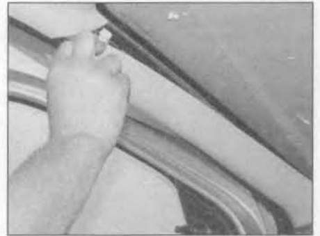
25.10 Carefully pull the front pillar trim panel away from the pillar to release the securing clips
