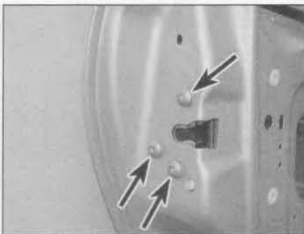
16.44 Undo the three screws (arrowed) securing the rear door lock mechanism to the door
