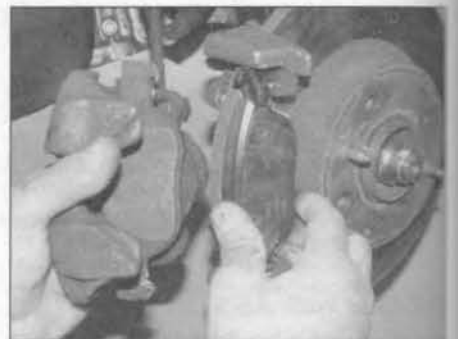
4.9b . . . and withdraw the outer brake pad from the mounting bracket – DOHC (16-valve) engine models
