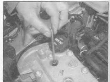
5.12c ... then insert the dowel rods
