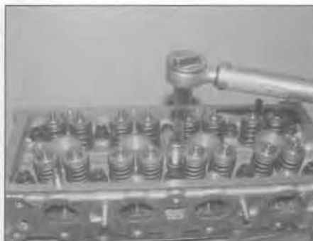
11.17b Tighten the cylinder head bolts to the Stage 1 torque setting . . .
