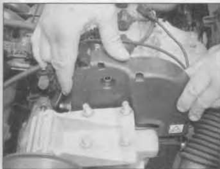
4.5 Lift the cover upwards, slip the TDC sensor wiring out of the groove, and remove the upper cover from the engine
