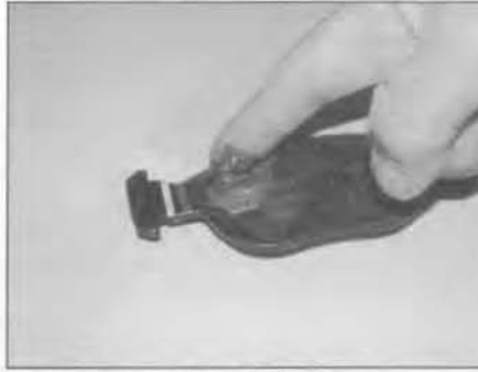
4.18 Sparingly apply high-temperature brake grease to the brake pad backing plates
