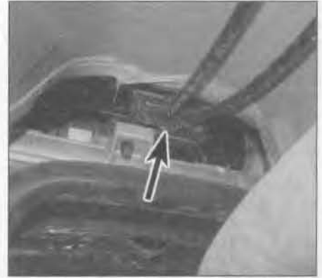
3.11 Release the selector cables from the support clip (arrowed) above the front subframe
