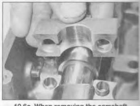
10.6c When removing the camshaft bearing caps, note the position of the long and short locating dowels
