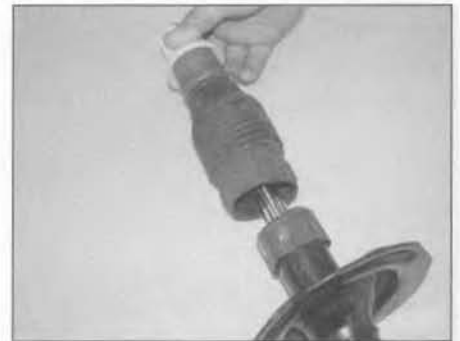
5.5 Release the dust cover from the strut body, then withdraw the dust cover and bump rubber
