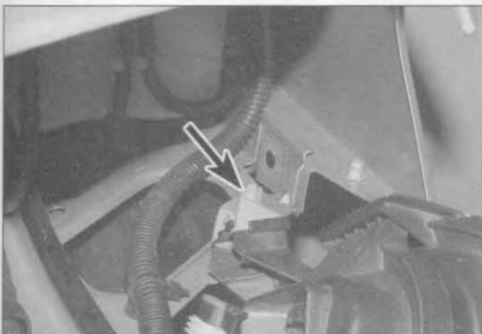
6.3b . . . then disengage the locating peg (arrowed) from the front wing
