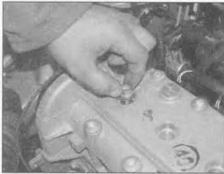
5.12a Screw the spark plug bodies of the home-made piston positioning tools into each spark plug hole ...
