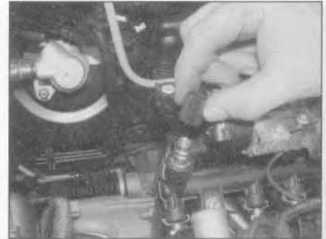
5.5 Withdraw the plastic cap from the top of the Schrader valve . . .
