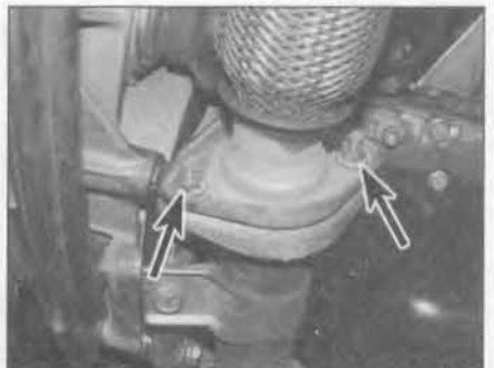
5.8 On models with air conditioning, undo the nuts (arrowed) and separate the exhaust manifold downpipe from the front pipe
