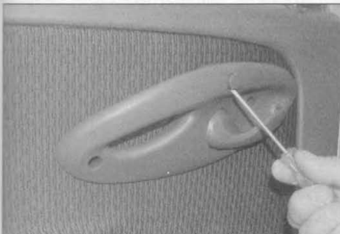
14.16a Lift off the trim caps and undo the retaining screws . . .
