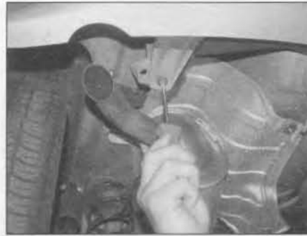
7.4 Undo the screws securing the rear bumper lower mountings to the brackets on the underbody
