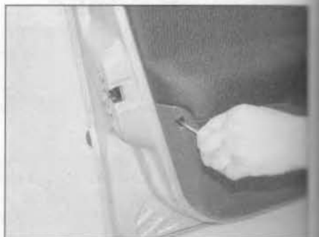
14.8b ... and undo the screw securing the rear of the trim panel to the door frame
