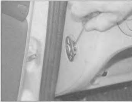
20.18a Prise out the passenger's airbag immobiliser switch from the facia . . .
