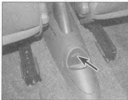
26.6a Undo the retaining screw (arrowed) . . .
