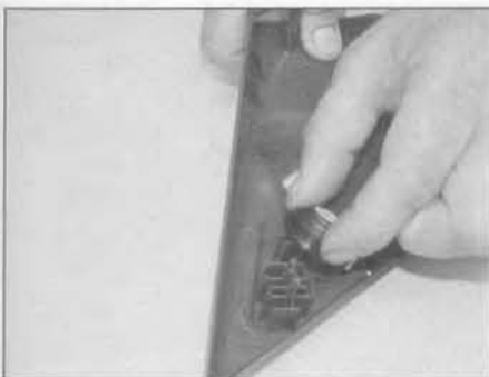
10.4b . . . and lift the speaker from the panel bracket
