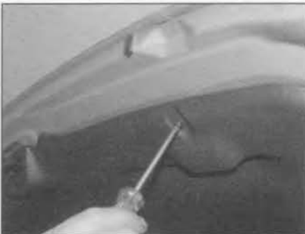
25.3 Undo the retaining screws securing the lower edge of the tailgate inner trim panel
