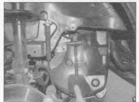
4.3 Remove the wheel arch liner panels for access to the crankshaft pulley
