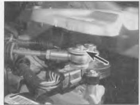
4.13 Extract the retaining clip (arrowed) and release the selector cable end fitting - automatic transmission models
