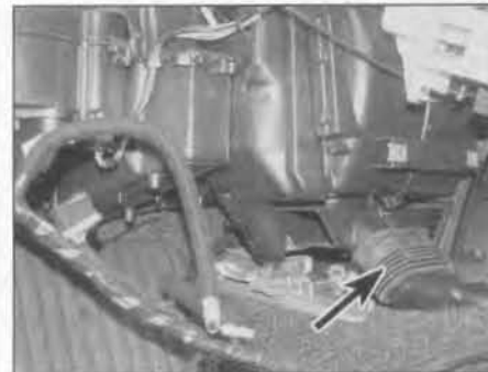
8.8 Remove the rubber sleeve (arrowed) between the heater and floor air ducts
