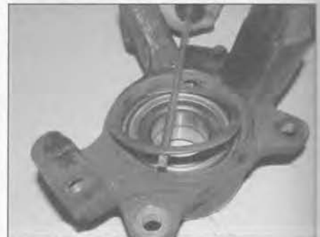
3.5 Extract the bearing retaining circlip from the swivel hub
