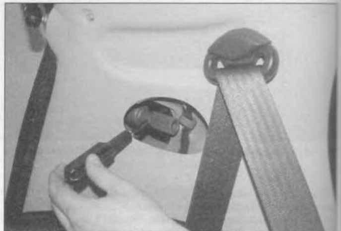
4.30 Unscrew the rear light cluster upper securing bolt using the screwdriver and special socket
