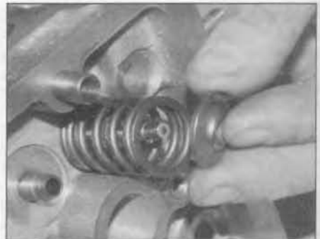
6.7a Release the compressor, and remove the spring retainer ...
