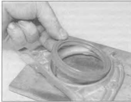
17.10b . . . locate the new oil seal in the housing . . .
