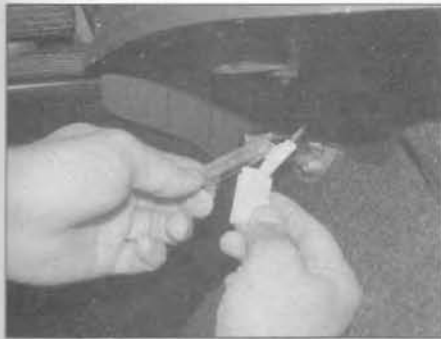
5.8a Open the bulbholder . . .
