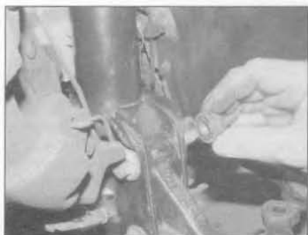
2.9a Unscrew the two nuts . . .
