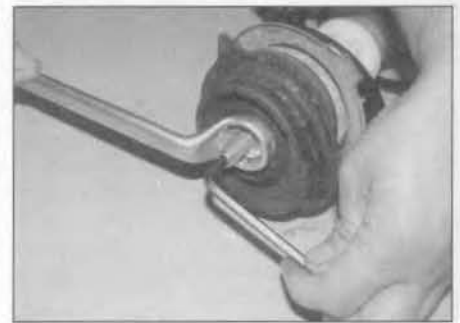
5.3 Unscrew the nut securing the strut piston rod to the upper mounting
