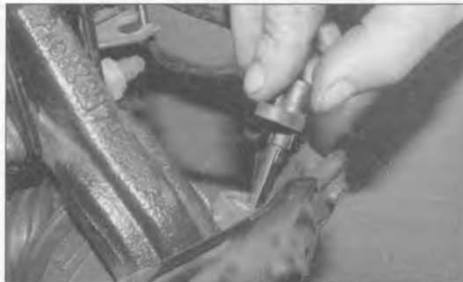
18.18 Unscrew the retaining bolt and withdraw the wheel speed sensor from the swivel hub
