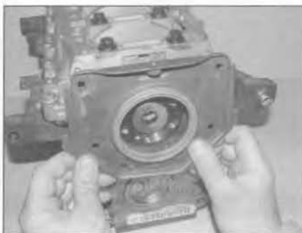
17.19 Lubricate the oil seal lips then locate a new rear oil seal housing into position – DOHC (16-valve) engines
