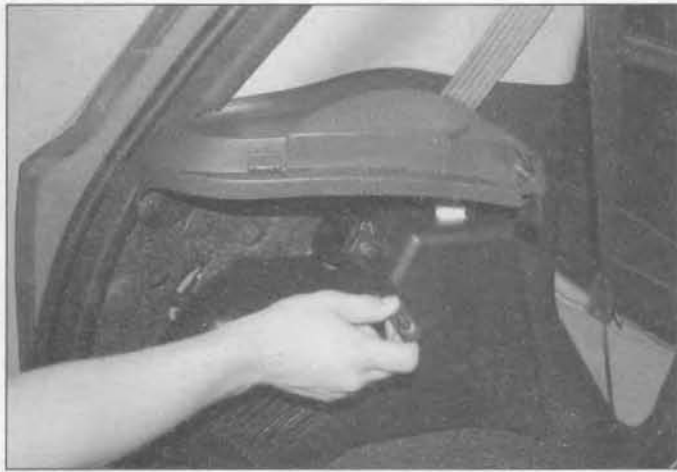
10.8 Undo the retaining screws, and remove the audio amplifier/loudspeaker unit
