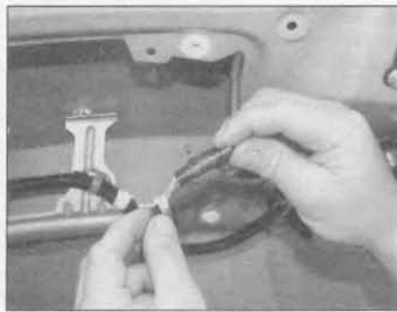
10.2 Disconnect the tailgate lock wiring connector ...
