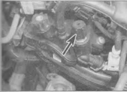
5.4a Fuel system depressurisation Schrader valve location (arrowed) on SOHC (8-valve) engines . . .
