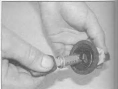
10.8b ... then withdraw the lock barrel from the lock cylinder
