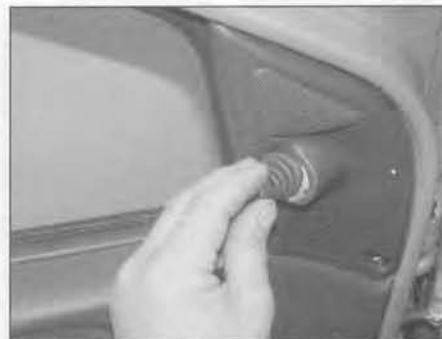
14.2a On manually-adjustable mirrors, prise the rubber cover off the adjustment lever
