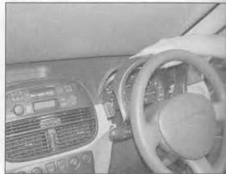
27.11b . . . then withdraw the surround from the facia
