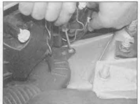
2.11 The cold air intake duct can be removed after undoing the end fitting retaining screw
