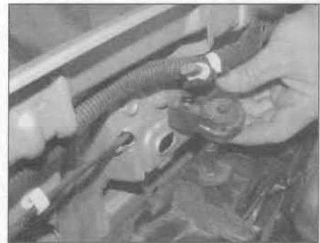
5.9b ... and remove the upper mounting bracket from the top of the fan shroud
