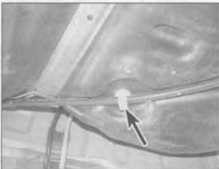
13.7c . . . and fuel tank (arrowed)
