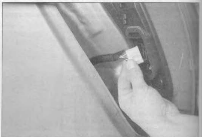
4.32 Withdraw the light cluster and disconnect the wiring connector
