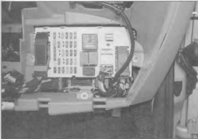
3.2 The main fuses are located in the fusebox under the fascia on the driver's side
