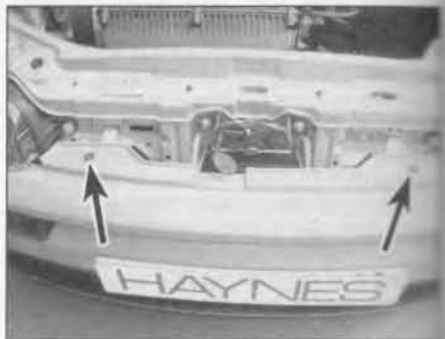
6.6 Undo the remaining two bolts (arrowed) from the upper edge of the bumper
