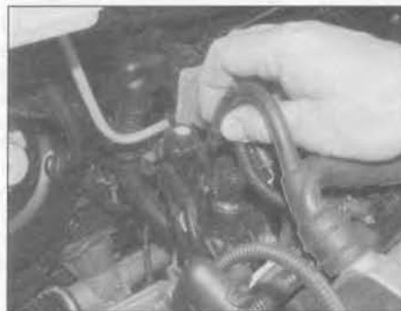
11.9 Disconnect the crankcase ventilation system hose from the right-hand side of the manifold – SOHC (8-valve) engines
