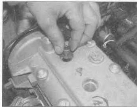
5.12b ... place a suitable washer or similar into the recess to keep the dowel rod vertical ...
