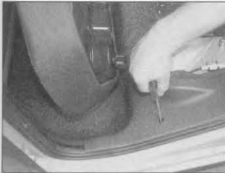
25.42 Undo the screws securing the side trim panel to the sill in the rear door aperture – 5-door models
