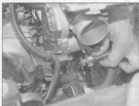
11.28 Release the clip and disconnect the coolant hose from the rear of the manifold – DOHC (16-valve) engines
