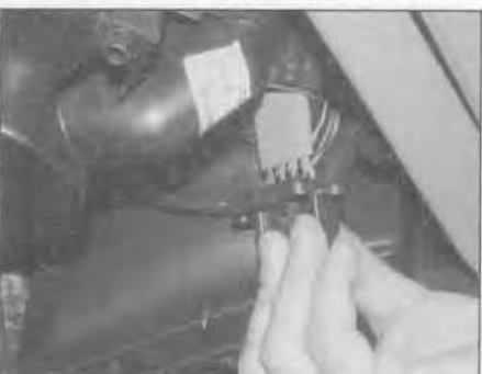
8.22 Undo the two screws and remove the blower motor resistor from the heater assembly
