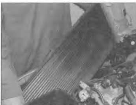
3.11 Carefully manoeuvre the radiator up and out of the engine compartment
