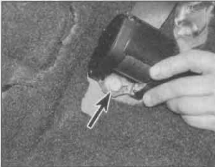
24.25 Rear seat belt inertia reel retaining bolt (arrowed) – 5-door models
