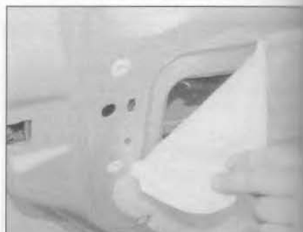
14.21 Carefully remove the plastic sealing sheet from the inside of the door
