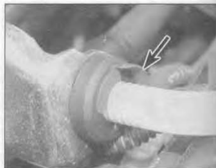
3.9 Accelerator outer cable retaining clip (arrowed)
