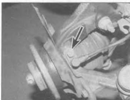
2.7b . . . then undo the retaining bolt (arrowed) and remove the sensor
