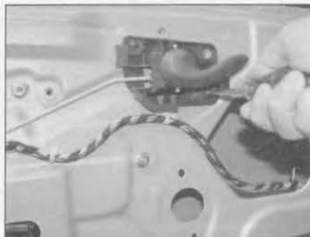
16.18 Undo the retaining screws and withdraw the interior handle from the door
