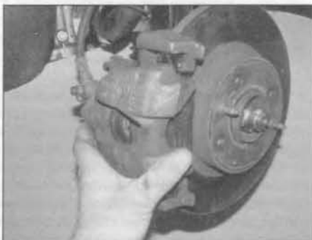
4.9a Lift off the brake caliper . . .
