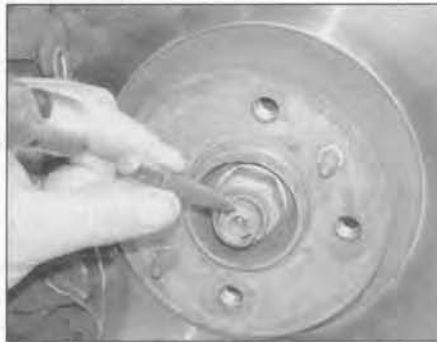
2.2 Tap up the staking securing the driveshaft retaining nut in position
