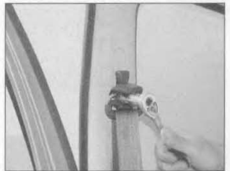
25.22 Undo the front seat belt upper anchor bolt . . .
