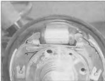
8.5a Correct fitted position of the brake shoe upper return spring ...
