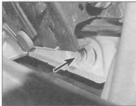
5.9a Undo the bolt (arrowed) below the bonnet lock ...
