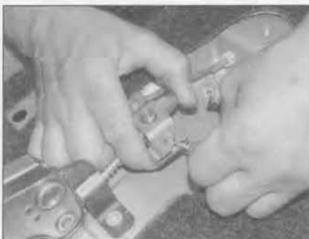
13.3 Disconnect the handbrake inner cable from the draw bar
