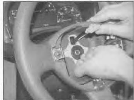
11.3 Lift off the protective seal over the steering wheel retaining nut
