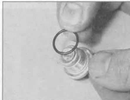
9.11 Renew the O-ring seals on the protective caps covering the cylinder head extension retaining bolts
