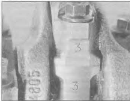
9.4 Connecting rod and big-end cap identification numbers
