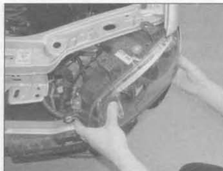
6.3a Withdraw the inner edge of the headlight unit from its location . . .
