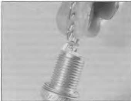
16.9 Adjusting a spark plug electrode gap
