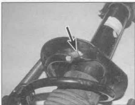
5.10 Fit the spring ensuring that the lower end locates in the spring seat recess (arrowed)
