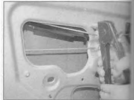
16.33 Refit the anti-theft partition and secure with new pop rivets
