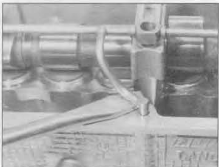
10.6a Prise out the feed stub of the camshaft lubrication pipe ...
