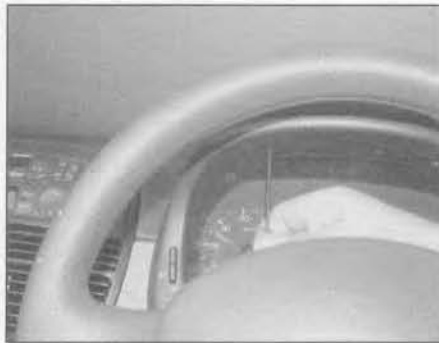
27.11a Undo the two upper screws . . .
