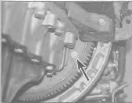
4.41 Torque converter retaining bolt (arrowed) accessible through the bellhousing opening - automatic transmission models
