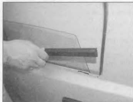
18.19 Carefully prise the rear door window aperture weatherstrip upwards and remove it from the door
