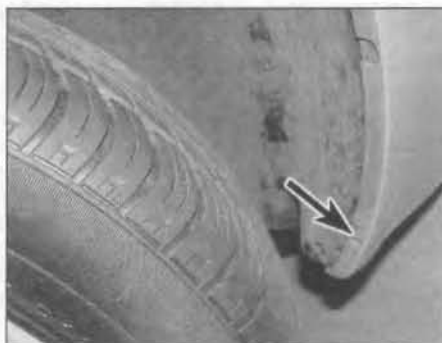
6.2b . . . and lower screw (arrowed) each side, securing the edge of the bumper to the wheel arch liner
