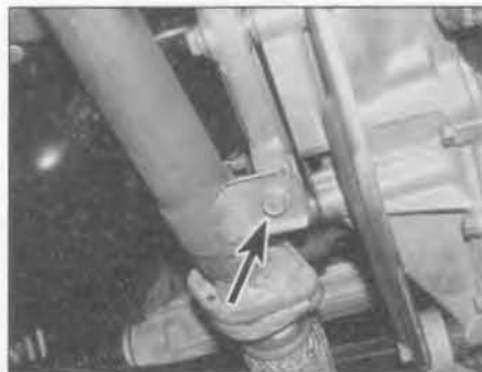
11.3 Undo the bolt (arrowed) securing the manifold downpipe support bracket to the transmission
