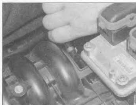
11.22 Release the clip and disconnect the vacuum hose from the rear of the manifold – DOHC (16-valve) engines
