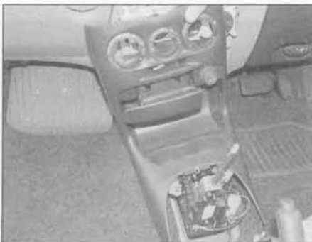
27.17 Disconnect the wiring connector, then withdraw the panel from the facia
