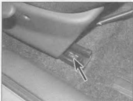
23.3 Front seat rail front securing bolt (arrowed) . . .
