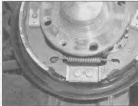
8.5b ... and lower return spring
