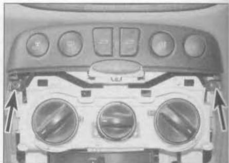
27.20 Undo the two lower screws (arrowed) securing the centre switch panel to the facia
