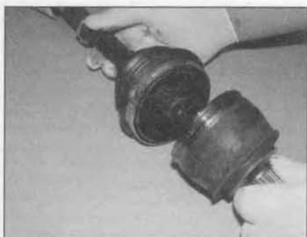
3.13a Engage the CV joint with the driveshaft splines . . .
