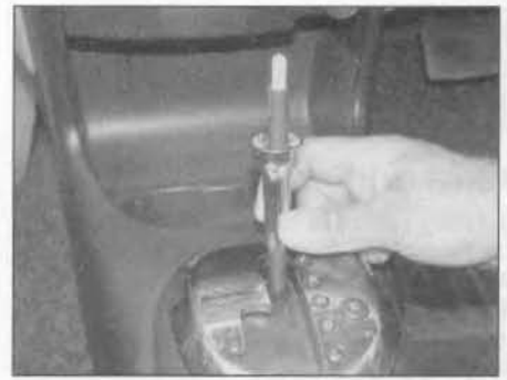
3.2c ... then remove the locking collar
