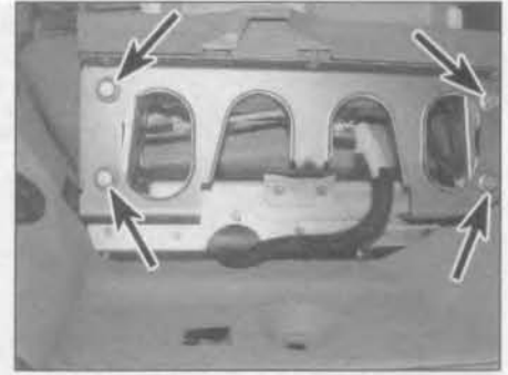
20.19 Undo the bolts (arrowed) securing the airbag assembly to the facia rail
