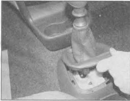
26.2a Carefully prise the base of the gear lever boot from its location . . .
