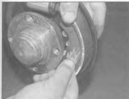
8.9a Remove the hold-down spring clip and pin from the trailing brake shoe . . .
