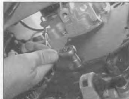
4.11 Undo the retaining bolt in the centre of the lower timing cover . . .
