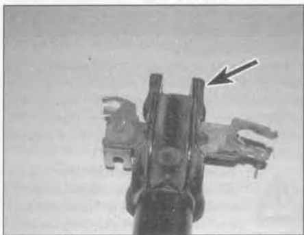
5.11b . . . is on the same side as the swivel hub mounting bracket (arrowed)
