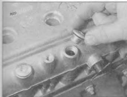
9.3 Unscrew the protective caps covering the cylinder head extension retaining bolts
