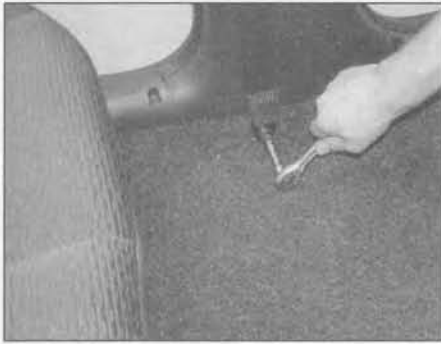
25.23 . . . and lower anchor bolt – 5-door models
