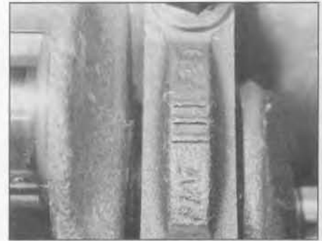
10.5 Main bearing cap identification markings – SOHC (8-valve) engines
