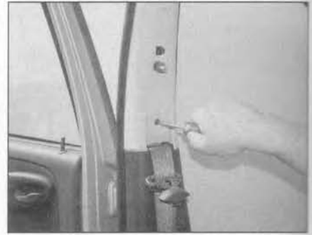
25.25 Undo the retaining screw at the base of the centre pillar trim panel upper section – 5-door models
