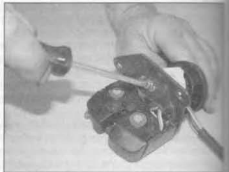
10.7 Undo the screw securing the lock cylinder to the tailgate lock body
