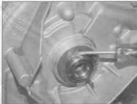
9.2 Carefully prise the crankshaft right-hand oil seal from the oil pump casing
