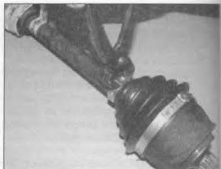
3.17 Slide the smaller clip over the gaiter, and secure it by compressing the raised portion
