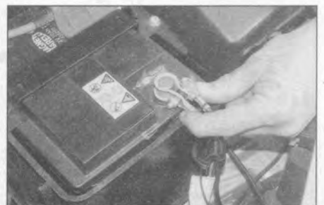
E Check the condition and security of the battery terminals.
