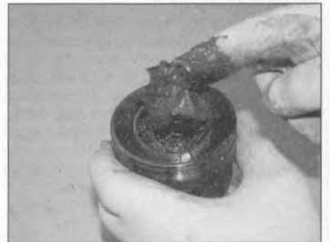
3.12 Pack the joint with the specified grease, then twist the joint to ensure all recesses are filled
