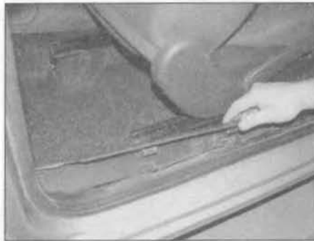
25.7 Carefully pull the panel away from the sill to release the securing clips
