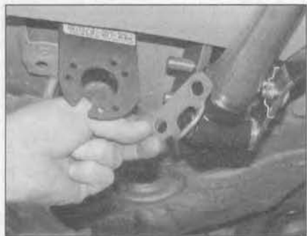
28.18a If the detachable towball is being fitted, position the receptor unit in the cross-bar, fit the bolts and safety chain plate ...
