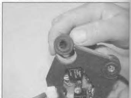
14.4b . . . and slide out the rubber bushes
