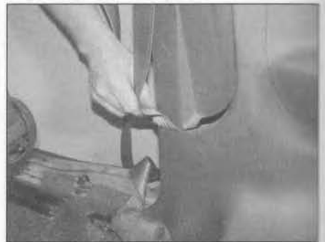
25.36 Slide the seat belt out through the incision in the panel – 3-door models
