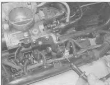
3.2b . . . and withdraw the outer cable from the rubber grommet on the mounting bracket
