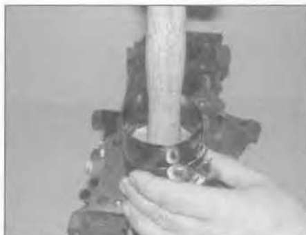
18.9 Tap the assembly into the cylinder using a block of wood or hammer handle
