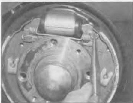
8.6a Detach the upper return spring ...
