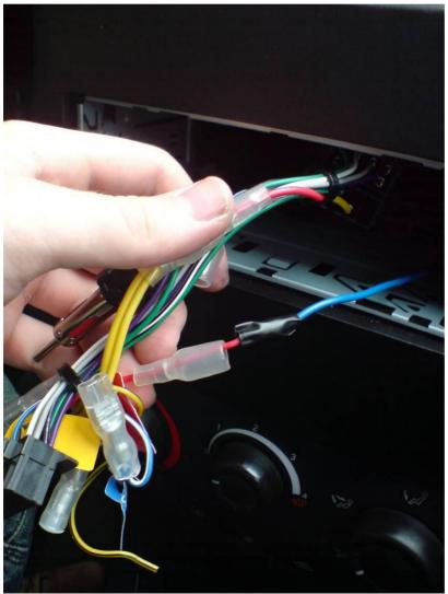
From the white plug from the car the only wires used are the red and black, the other two stripey ones were used for the CAN system. The red is live and the black in earth, this red connects to the red
