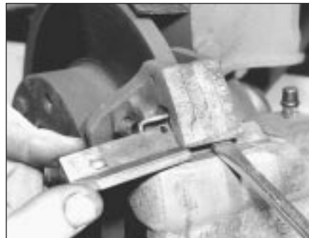
14A.2B Front brake locking block orientation with inboard retaining clip
