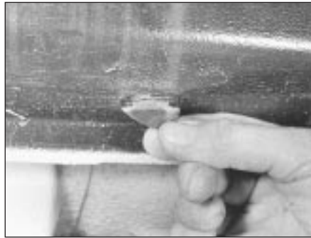
2.4B Sill drain with non-return valve
