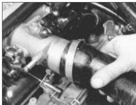
9C.31A Disconnecting the throttle valve housing intake duct
