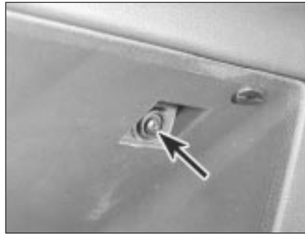
22.5A Fascia fixing screw inside glovebox
