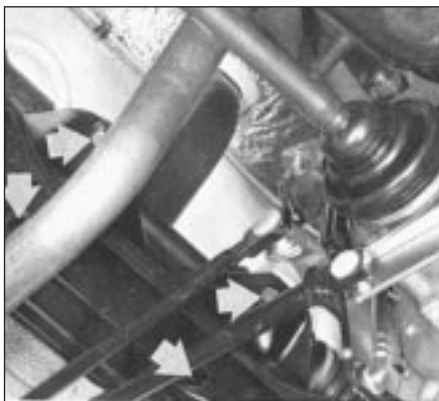
Fig. 11.6 Steering rack mounting bolts (Sec 7)
