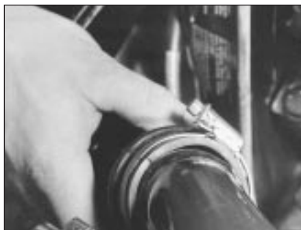
9C.55A Disconnecting the duct from the air cleaner
