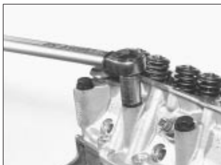
7B.121A Tighten main cylinder head bolts to specified torque . . .
