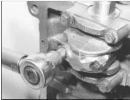
5B.99 Tightening a big-end cap bolt
