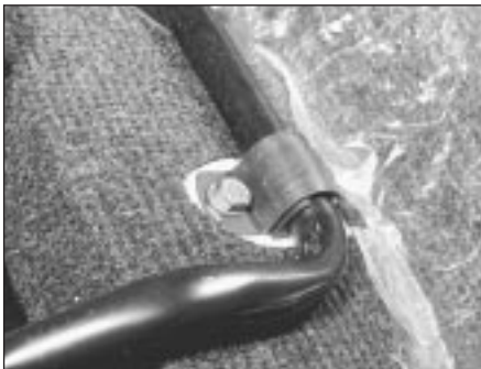
19.1 Front seat mounting clamp
