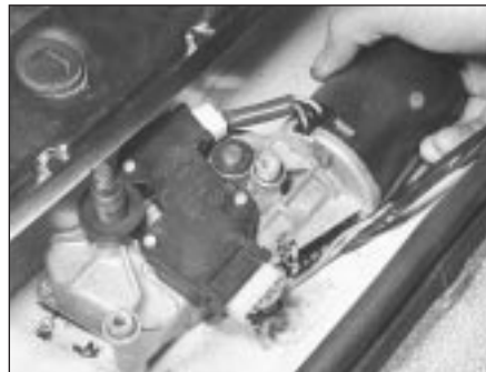
25.5B Removing windscreen wiper motor
