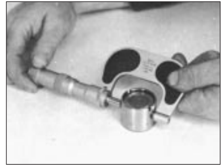
Fig. 13.8 Checking a cam follower for ovality - 999 and 1108 cc engine (Sec 5C)
