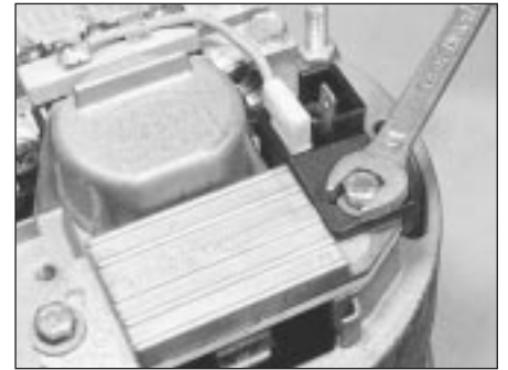
5.3A Alternator brush holder bolt
