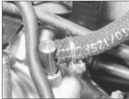
44.21B Brake servo hose at manifold
