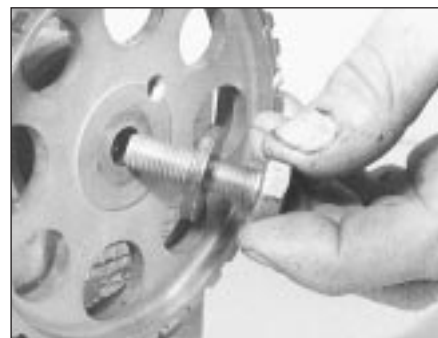
5B.22B Camshaft sprocket bolt and washer
