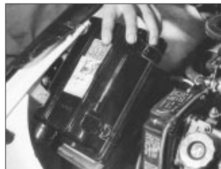
9C.27A Removing the air cleaner lid
