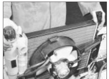
7.4B Removing radiator/fan assembly
