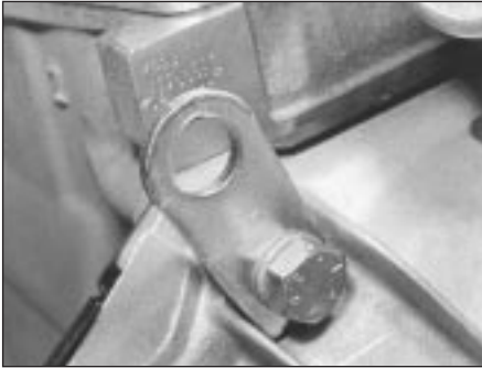
44.2 Lifting lug at bellhousing bolt
