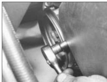
5B.6 Timing cover lower fixing bolt removal
