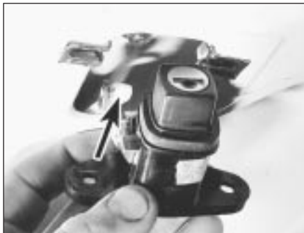
17.13 Tailgate handle link rod (arrowed)
