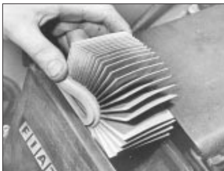
9A.4B Air cleaner element on the 999 cc model
