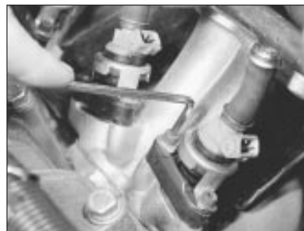
9C.80A Extracting a fuel injector screw
