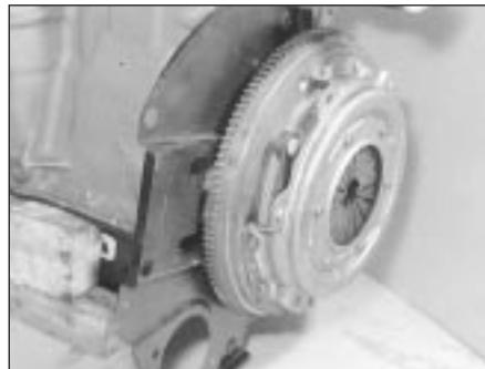
42.27 Engine rear plate nut
