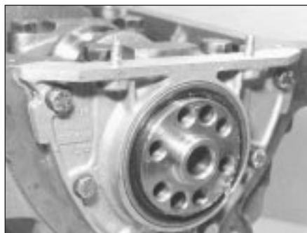
42.7C Rear oil seal carrier
