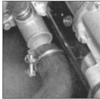
Fig. 1.13 Coolant hose at rear of coolant pump (Sec 13)
