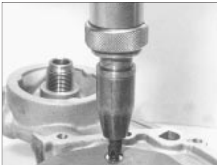
5B.73 Removing the oil pump rear cover plate screws
