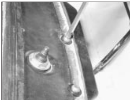
25.4 Removing windscreen wiper motor mounting screws
