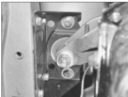
5C.32 Right-hand engine mounting brackets on body and engine
