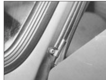
15.108B Pillar lower screw for aerial
