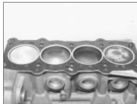
5B.50A Cylinder head gasket
