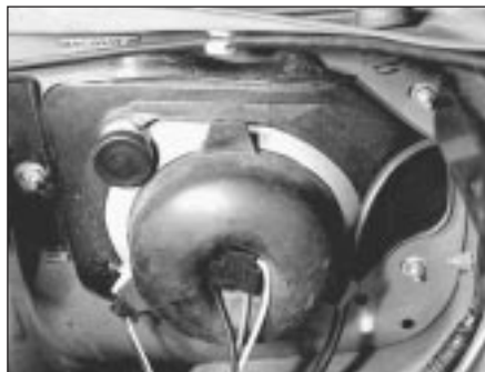
15.28 Headlamp unit fitted to the 1372 cc ie model
