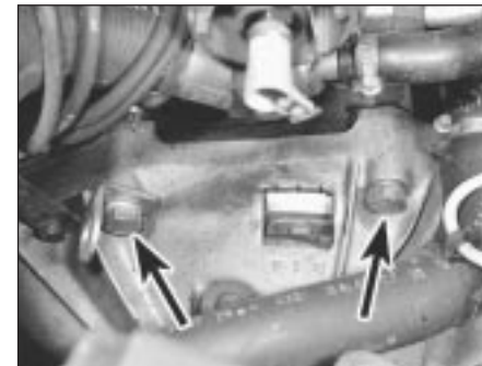
12B.36 Transmission upper retaining bolts. Note bracket under the left-hand bolt
