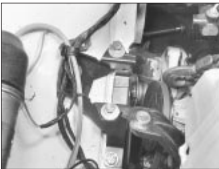
44.8C Right-hand engine mounting brackets
