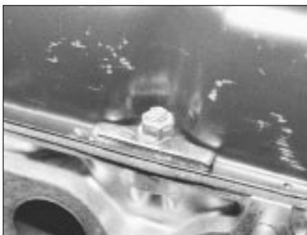
20.30 Rocker cover nut and thrust plate
