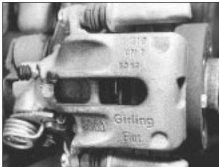
14B.23 Rear brake pad inspection aperture
