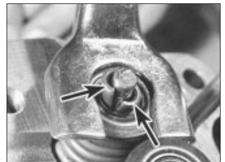
17.19 Fitting split collets
