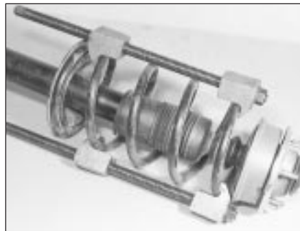
3.6 Spring clamps in position
