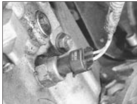
7C.14 Reversing light switch and lead
