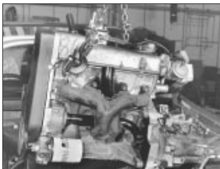
5C.34 Lifting out the engine and transmission
