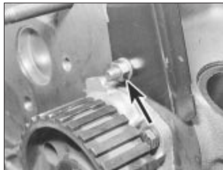
42.24B Belt cover mounting stud
