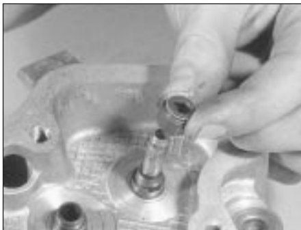
7B.130C . . . locate stem oil seal . . .
