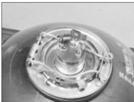
16.2A Headlamp bulbholder spring clips
