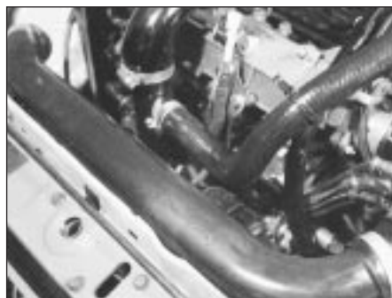
9C.55D Air cleaner metal duct over radiator
