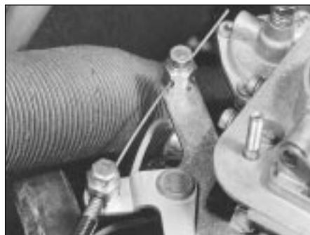
9B.37C Choke cable connection on the Weber 30/32 DMTE carburettor
