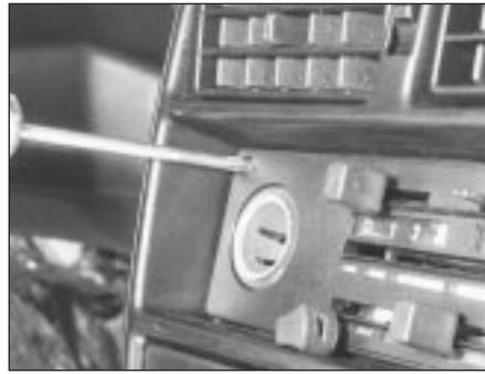
12.6A Heater control panel screw
