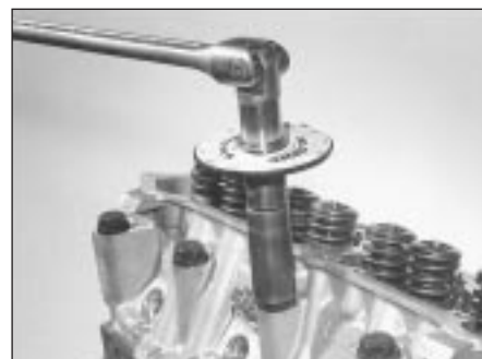
7B.121B . . . and then through the specified angle
