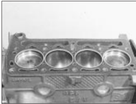
7.20 Cylinder head gasket
