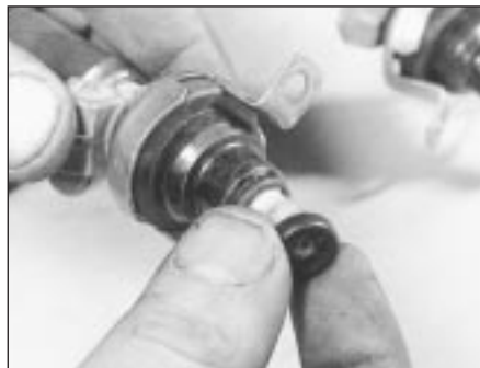
9C.95B Fuel injector small seal
