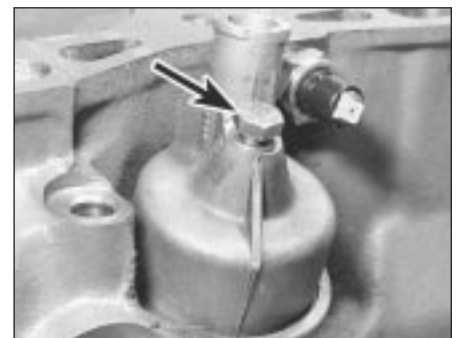
42.16B Crankcase breather and retaining bolt
