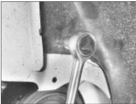
10.4A Unscrewing wing shield screw
