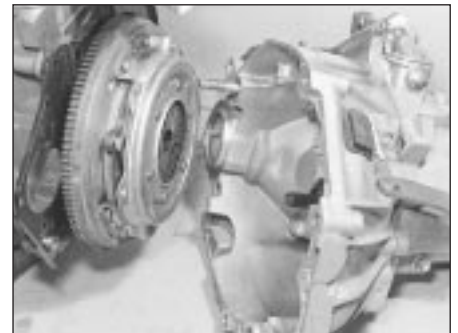
44.1 Offering transmission to engine
