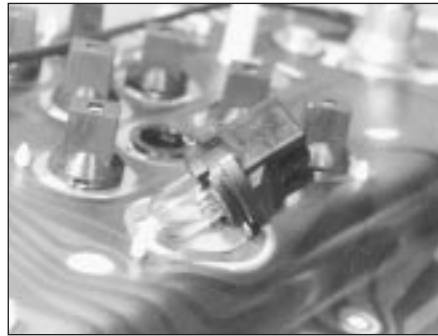
20.3 Instrument panel warning lamp
