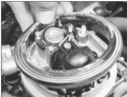
9D.39 Removing the filter seal from the injector unit
