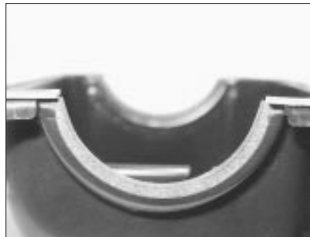
8.4 Sump pan sealing strip
