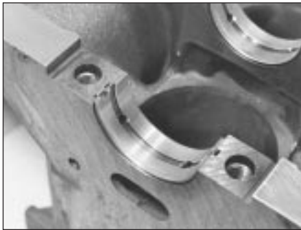
5D.2 Main bearing shell in crankcase
