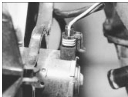
5C.19B Radiator fan motor wiring connector
