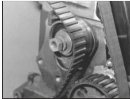
28.8 Slipping timing belt onto tensioner pulley
