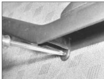
11.1A Removing an armrest screw
