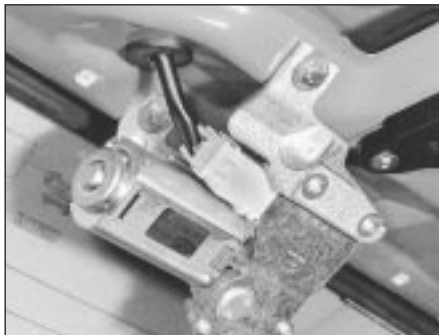
15.106 Tailgate wiper motor - later model
