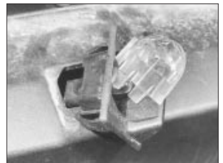
19.12 Rear number plate lamp withdrawn
