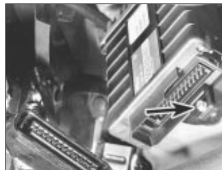
9D.58B . . . for access to the ECU retaining screw (arrowed)
