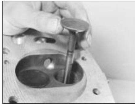
39.5 Removing a valve
