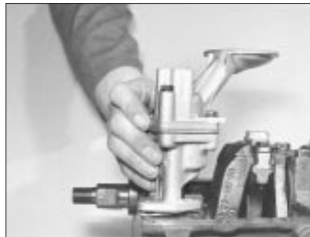
10.4 Fitting the oil pump
