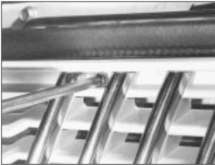
17.19A Extracting a radiator grille screw
