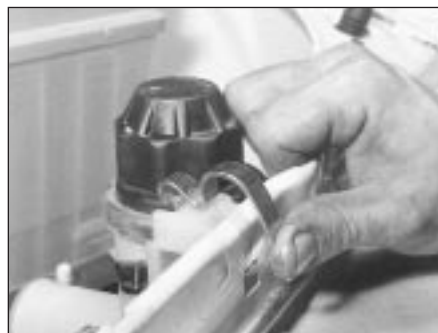
7.4A Radiator fixing clip
