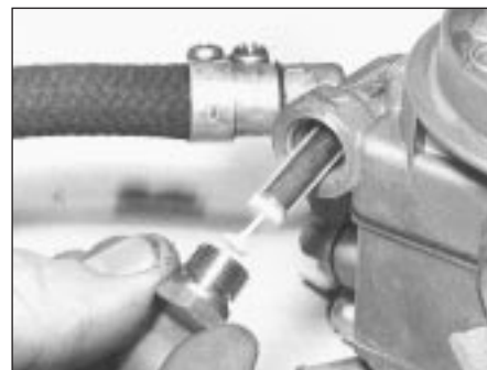
9B.22 Fuel filter removal from the Weber 32 TLF carburettor
