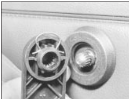
11.4 Window regulator handle removed
