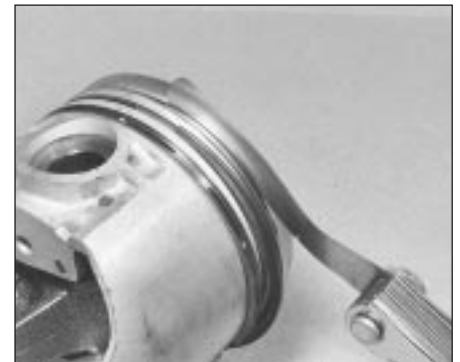
18.24A Checking piston ring groove clearance
