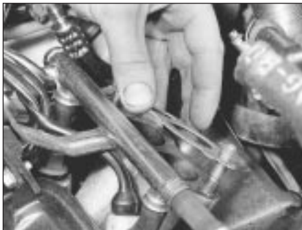
9C.95D Inlet pipe stub gasket
