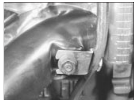
21.5B Dipstick guide tube support
