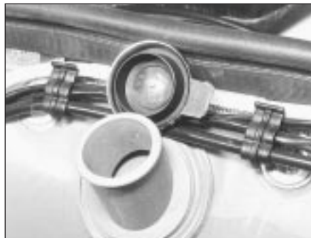
28.1 Washer fluid reservoir
