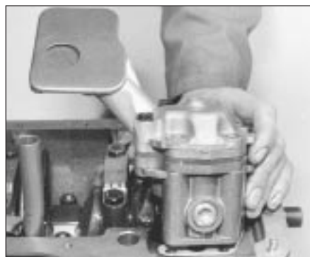
42.13 Locating oil pump and gasket
