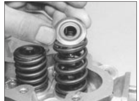
39.4A Valve spring cap
