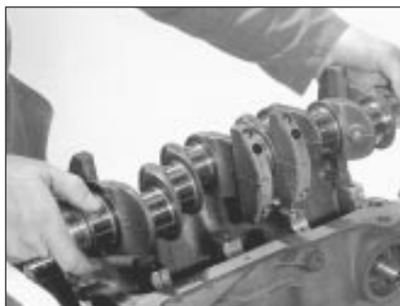
7D.10 Lower the crankshaft into position
