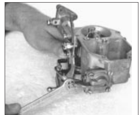
Fig. 3.17 Adjusting accelerator pump rod (Solex C32 DISA 11) (Sec 10)
