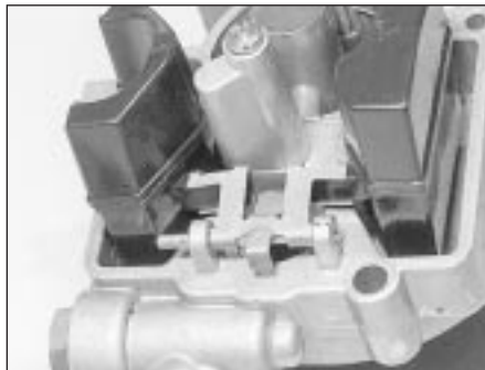
9B.26A Floats and pivot pin arrangement on the Weber 32 TLF carburettor
