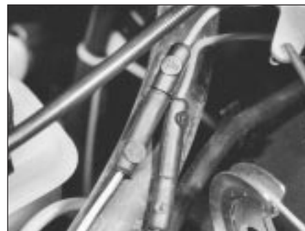
9B.37E Carburettor lead connectors on the Weber 30/32 DMTE carburettor
