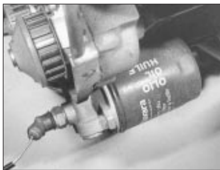
5C.18 Oil pressure switch
