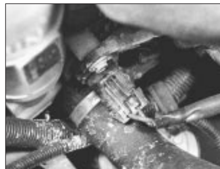
8C.21B Cooling fan switch wiring connector
