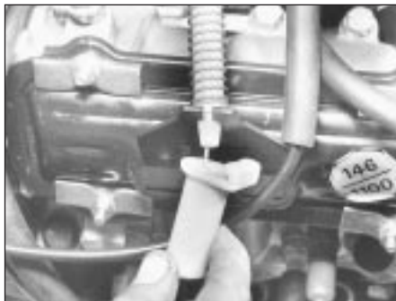
17.4 Throttle cable sleeve and bracket
