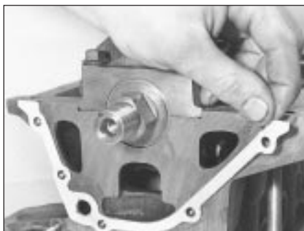
5D.12A Oil pump gasket
