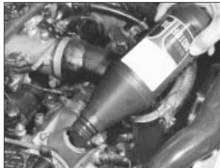
6C.27 Filling the engine with oil
