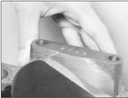
20.6 Fitting a main bearing cap
