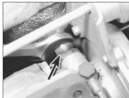
9F.18A Releasing turbocharger coolant inlet union (arrowed)
