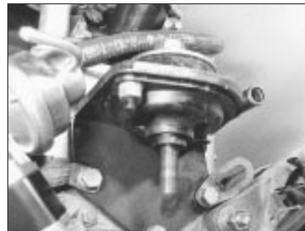
13.25 Right-hand engine mounting
