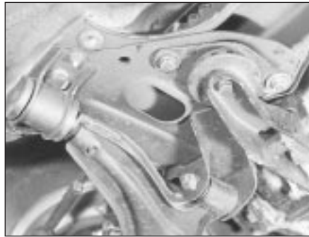
6.3 Track control arm inboard fixing
