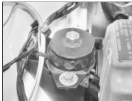
44.8D Right-hand mounting bolted up
