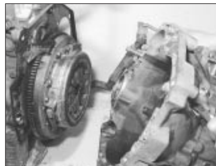
5C.39 Separating the engine and transmission
