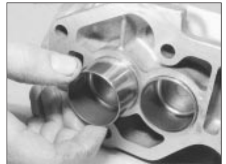
39.10 Cam followers fitted to camshaft carrier
