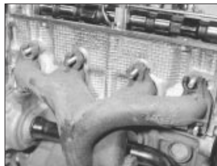
5D.31 Exhaust manifold
