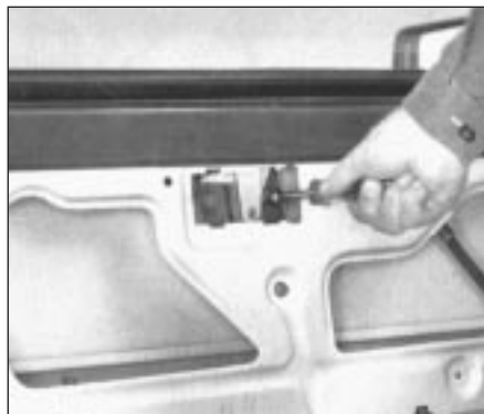
Fig. 12.6 Door glass mounting screw (Sec 12)
