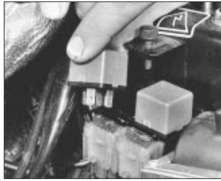
9D.27 Fuel pump relay removal
