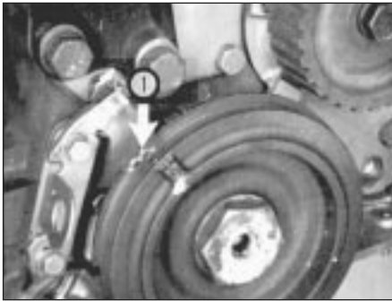
Fig. 1.28 TDC marks (1) at front of engine (Sec 28)
