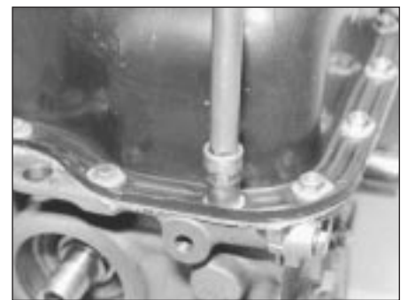
42.14 Tightening sump pan bolt
