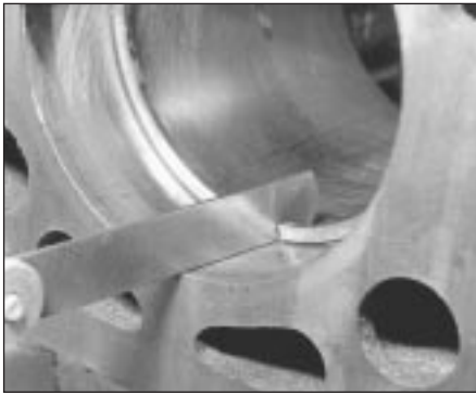
18.24B Checking piston ring end gap
