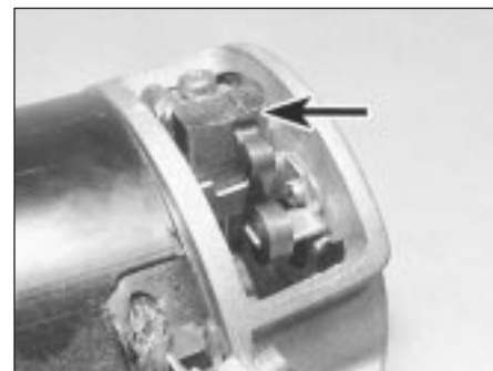
9.4 Starter motor brush partly withdrawn
