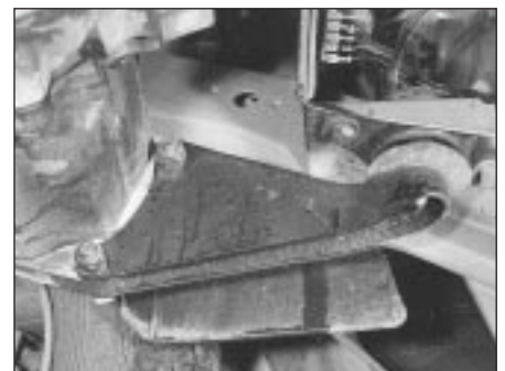
5C.31B Left-hand engine mounting and bracket
