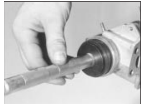
7B.97B Inserting the new camshaft front oil seal
