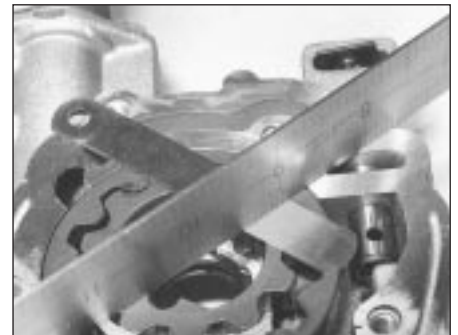
5B.74B Checking the oil pump gear endfloat
