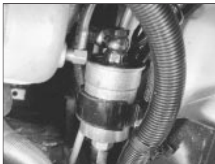
9C.25 Secondary fuel filter
