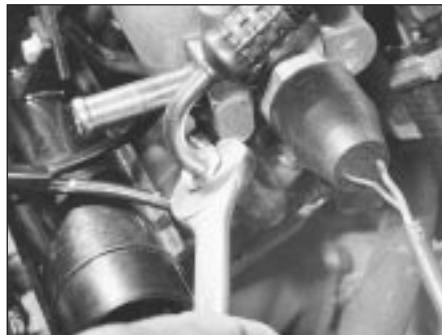
9C.75 Disconnecting the fuel delivery hose union
