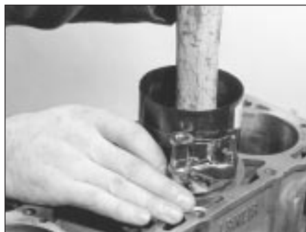
7B.194B Tapping a piston into its bore
