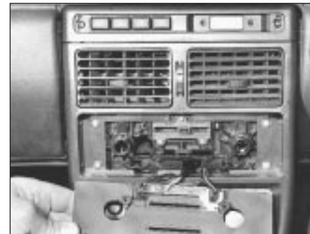
15.69B . . . and withdraw the heater control panel
