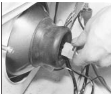
16.1 Headlamp plug and rubber cover
