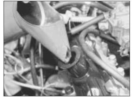
2.3B Topping up engine oil (1116 cc)
