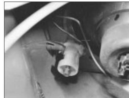
15.29 Headlamp beam adjuster on the 999 cc Turbo ie model
