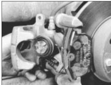
14B.26 Withdrawing the rear brake caliper
