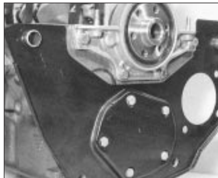
20.12 Engine rear plate
