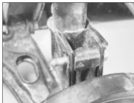
3.3 Strut clamp bolt
