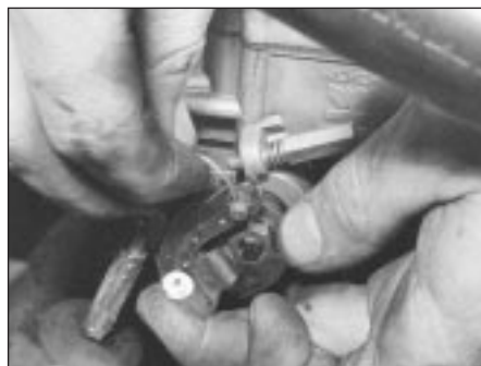
5B.32 Disconnecting the throttle cable
