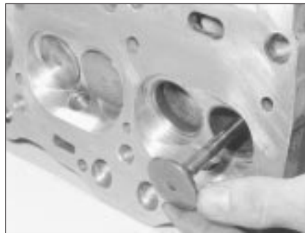
7B.130B Valve assembly - 1372 cc engine; insert valve into guide . . .
