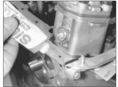
7B.165 Apply sealant to the front oil seal housing/cylinder block joint
