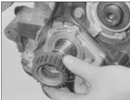
7B.47 Refitting the crankshaft sprocket
