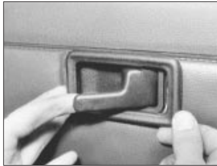
11.3A Removing remote control handle escutcheon
