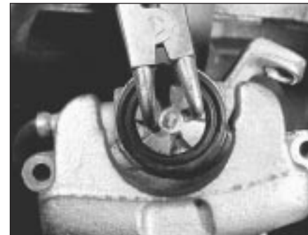
14B.28 Rotating a rear caliper piston
