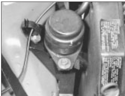
7C.36A Engine right-hand mounting
