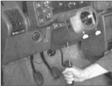
Fig. 10.2 Removing steering column shroud screws (Sec 5)
