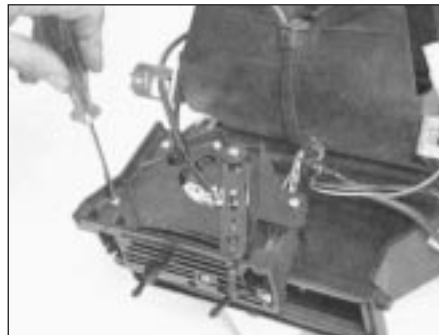
Fig. 2.9 Control lever platform screw (Sec 13)
