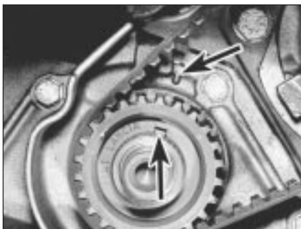
7B.50 Crankshaft at TDC with key and timing mark aligned (arrowed)
