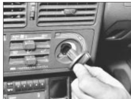
8D.15 Pull free the heater/fresh air and blower control knobs
