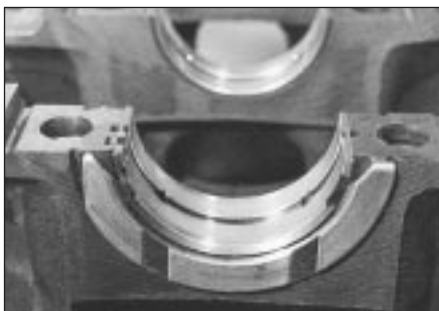
5D.3 Crankshaft thrust washer at centre bearing
