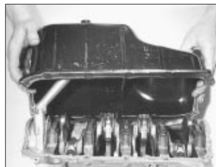
5C.60A Removing the sump pan
