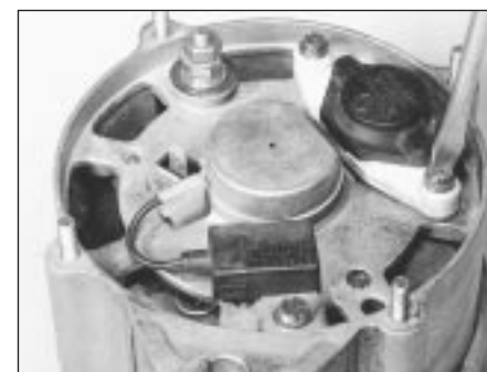
15.16A Extracting the alternator brush holder screw
