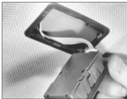
15.86 Remote control receiver unit removal
