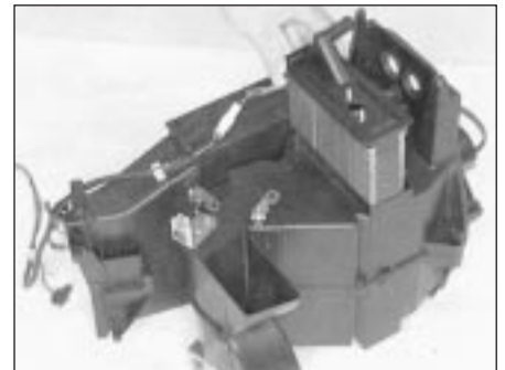
Fig. 2.10 Withdrawing heater matrix (Sec 13)
