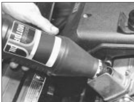
7A.11 Topping up the engine oil level - 1372 cc engine
