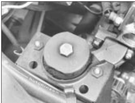
5B.107C Right-hand engine mounting
