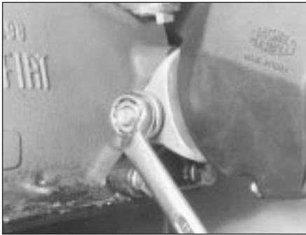
4.2A Alternator mounting
