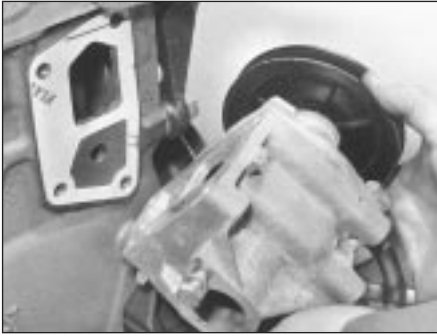
9.21 Fitting coolant pump (1116 cc engine)
