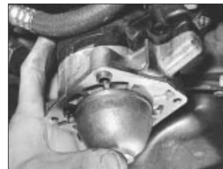
15.23A Starter motor removal from the 1301 cc Turbo ie engine
