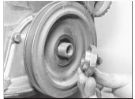
42.21 Crankshaft pulley and nut
