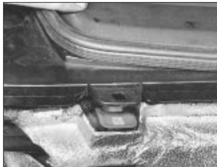
15.96A Release the air grille from its fixing points . . .
