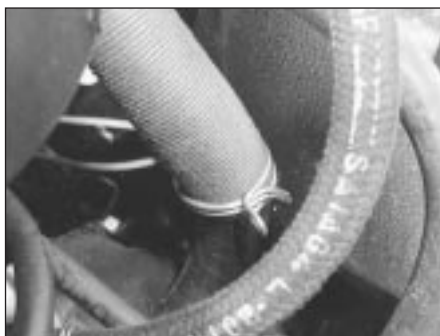
2.1 Air cleaner hot air intake
