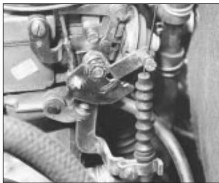
5C.12 Choke cable connection at carburettor
