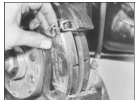
3.8A Disc pad and anti-rattle spring
