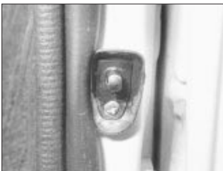
12.1 Courtesy lamp switch
