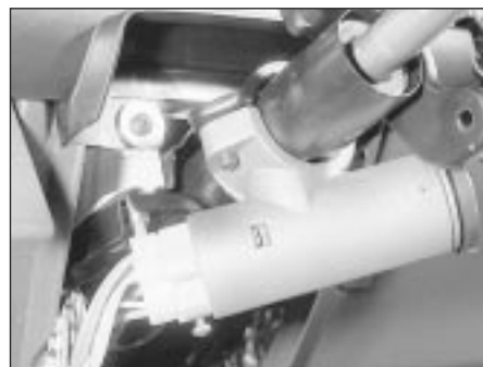
12.2 Ignition switch and lock
