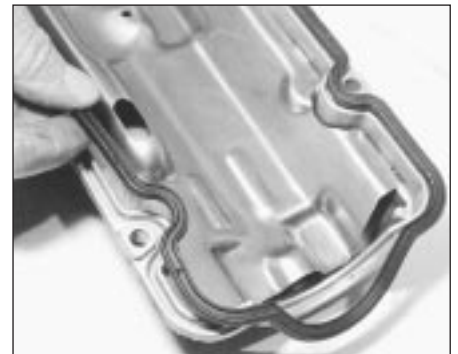
5B.26B Camshaft cover gasket
