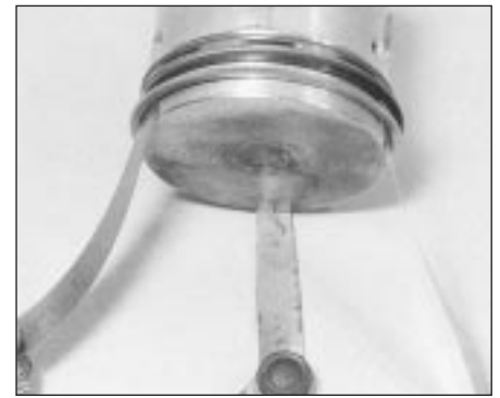
18.20 Using feeler blades to fit piston rings
