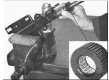
Fig. 10.4 Renewing steering shaft bushes (Sec 5)
