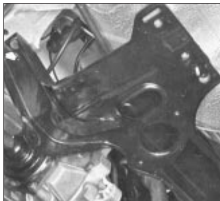
Fig. 11.7 Front crossmember bolts (Sec 7)
