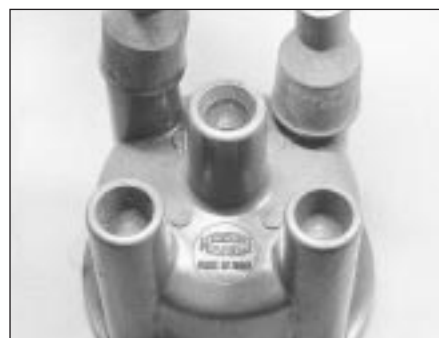
11.7 Distributor cap HT lead markings
