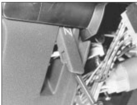
18.3 Extracting choke control lever screw
