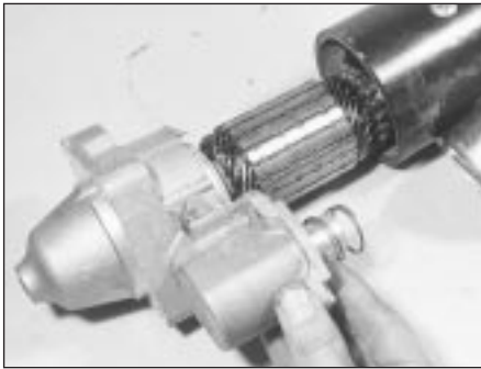
9.8 Starter motor dismantled
