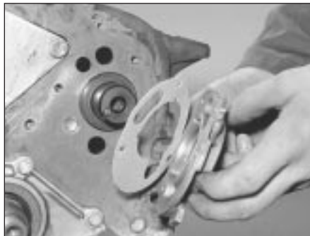
7C.55A Refit the auxiliary shaft cover with a new gasket . . .
