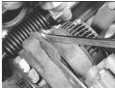
8C.53 Tightening the alternator adjuster nut
