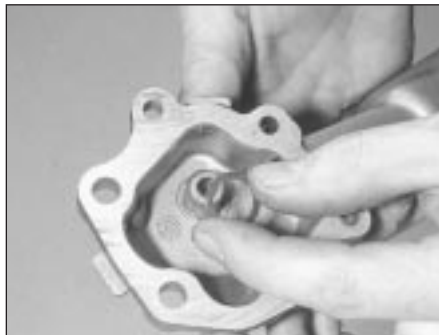
7B.180B Locate spring seat over boss within pump cover . . .
