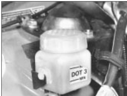
11.7A Clutch hydraulic fluid reservoir showing MIN and MAX markings
