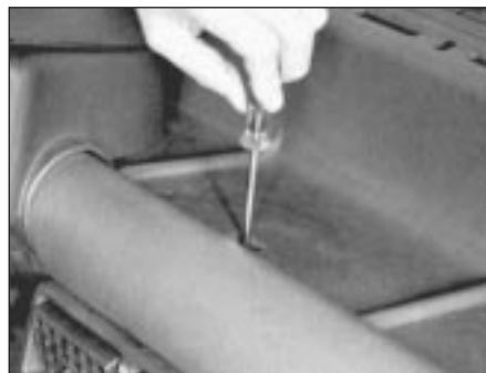
Fig. 2.8 Extracting heater upper fixing screw (Sec 12)
