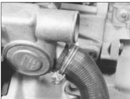
7.3B Radiator hose to thermostat housing
