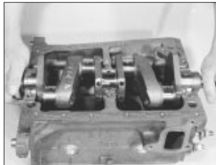
20.4B Lowering crankshaft into position
