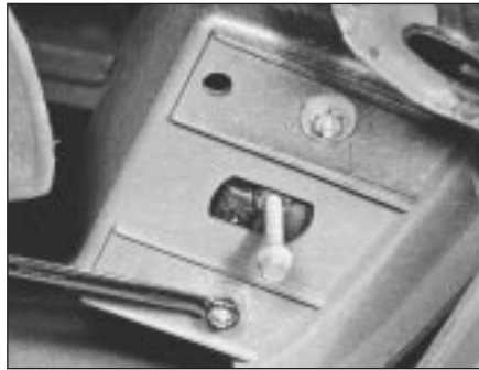
15.37A Undo the retaining bolts . . .
