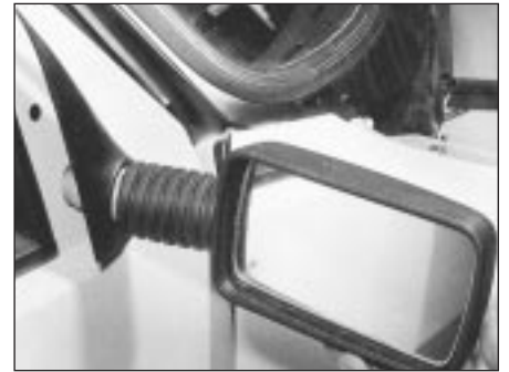
24.4 Withdrawing exterior mirror and trim plate
