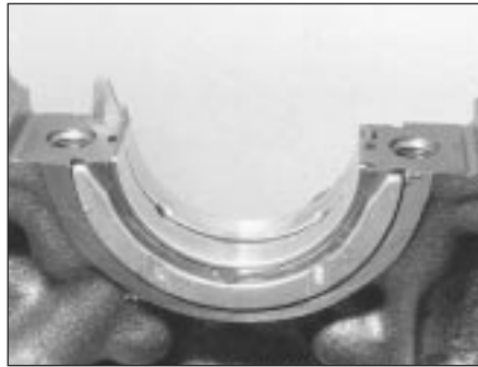
42.2 Crankshaft thrust washers
