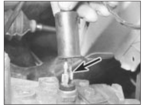
44.22A Reversing lamp switch on transmission
