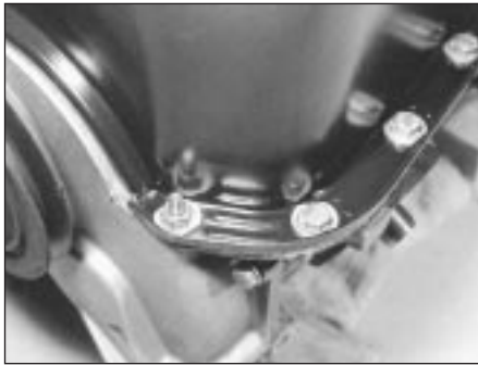
8.7B Sump pan nut, bolts and washers
