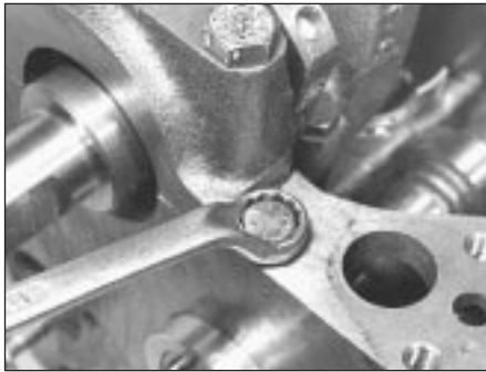
20.17 Camshaft front bearing lockscrew
