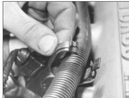
9C.77 Wiring loom clip and bracket
