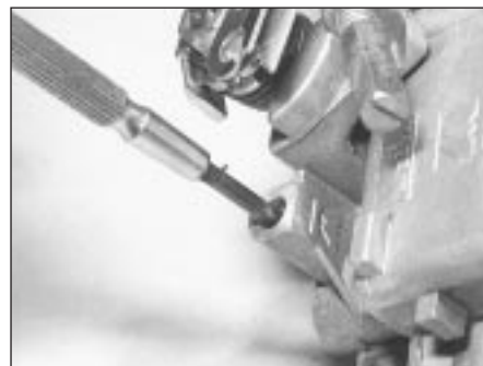
9B.9 Mixture adjustment - Weber 32 TLF carburettor
