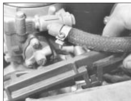
5B.20A Camshaft cover HT lead clip
