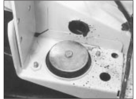
44.8B Left-hand engine mounting
