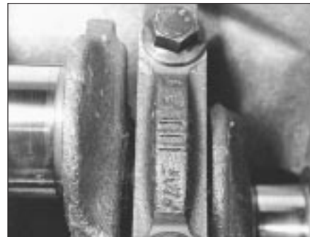
5C.66 Main bearing cap markings
