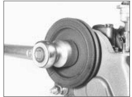
20.23 Tightening crankshaft pulley nut
