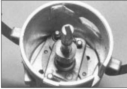
7.13 Marelli distributor centrifugal weights and springs
