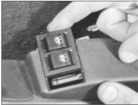
17.34A Armrest electric window switches
