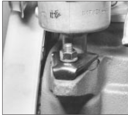
4.5 Distributor clamp plate nut
