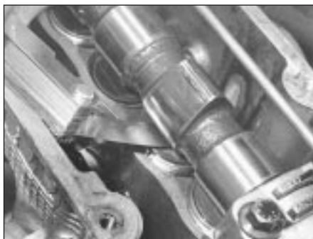
5B.1A Checking a valve clearance
