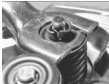
39.2 Valve spring compressor and split collets
