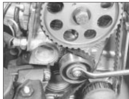
5B.9 Releasing the timing belt tensioner nut
