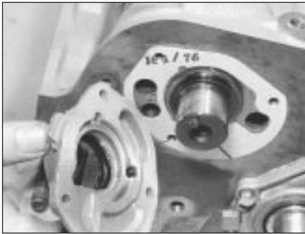
42.10A Auxiliary shaft end plate and gasket
