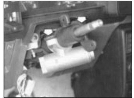
Fig. 10.9 Steering column lock shear bolts (arrowed) (Sec 9)
