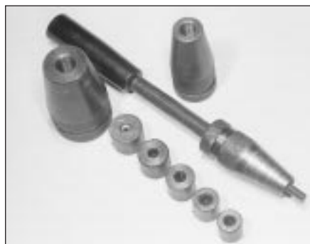
Clutch plate alignment set
