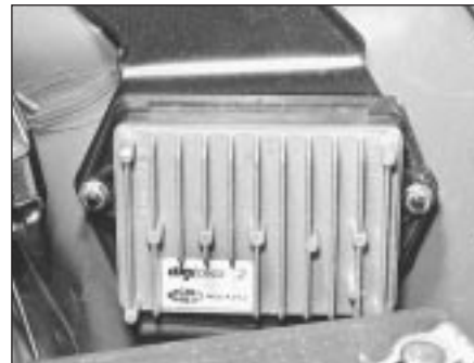
10.68 ECU location on the 1372 cc ie engine
