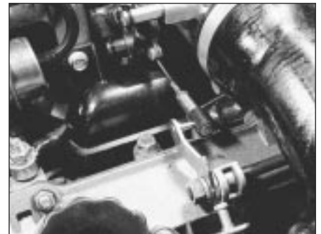
9C.99B Throttle cable (secondary section) and cross-shaft
