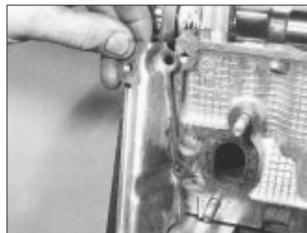
5D.20 Fitting the timing belt rear cover
