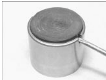
26.2 Removing a shim from a cam follower
