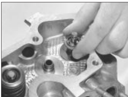
7B130F . . . locate the spring seat . . .
