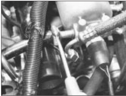
9C.88A Disconnecting the supplementary air valve hose from the inlet manifold
