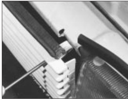
17.19B Prising down a radiator grille clip
