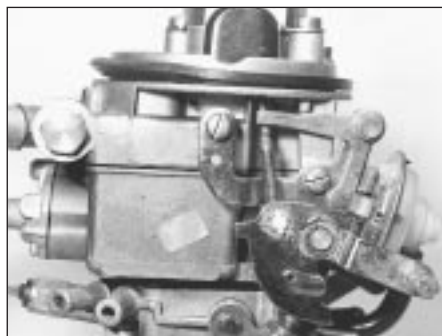
9B.2B Weber 32 TLF 4/250 carburettor from choke linkage side
