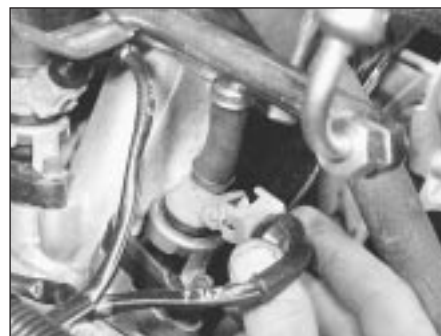
9C.81C Injector wiring plug refitting
