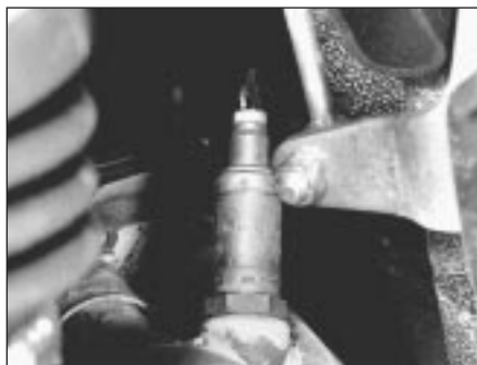
9D.69 Lambda sensor in exhaust downpipe
