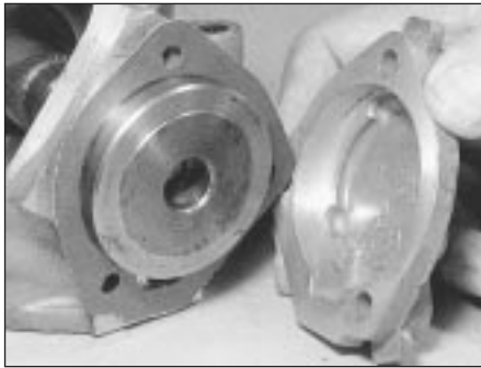
27.13A Removing camshaft end cover
