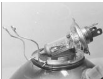
16.2B Headlamp halogen type bulb
