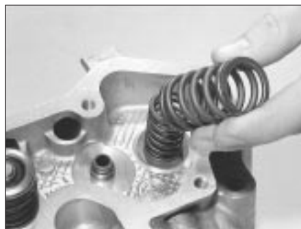
7B.130H . . . the outer spring . . .
