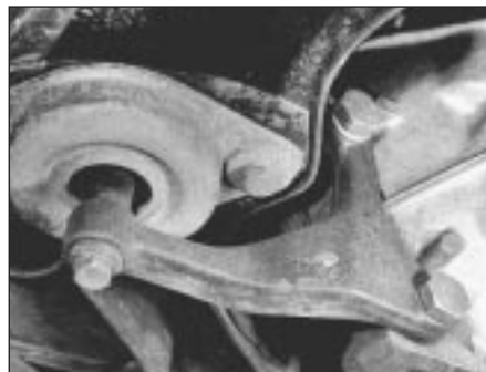
7C.36B Transmission rear mounting
