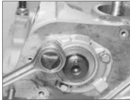
42.10B Tightening auxiliary shaft end plate bolt
