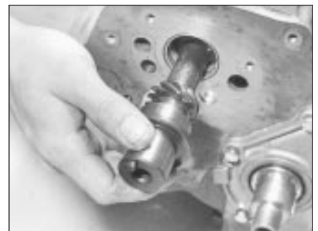
42.9 Fitting the auxiliary shaft
