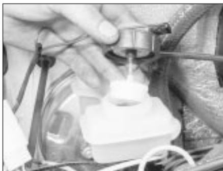
2.3 Fluid reservoir cap and float for warning switch
