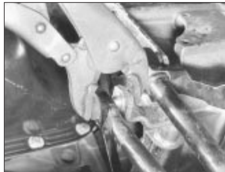
44.14 Connecting a gearchange rod ball cup
