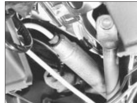
11.12 Clutch master cylinder and hydraulic pipe connections
