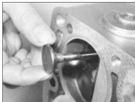
17.17B Inserting a valve into its guide
