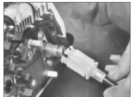
23.2 Speedometer cable connector at head
