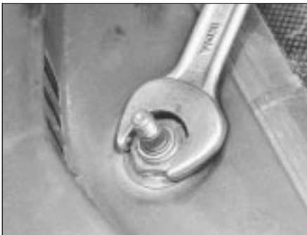
15.95 Unscrewing the wiper pivot nut
