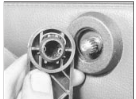
11.7 Window regulator handle ready for fitting
