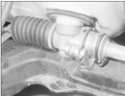
6.4 Steering rack housing at pinion end
