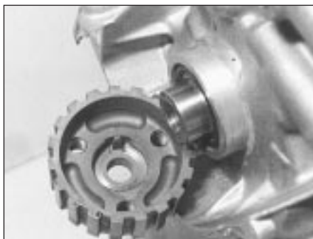
5D.16A Crankshaft sprocket showing integral key
