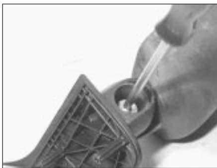
17.8 Extracting the mirror balljoint screw
