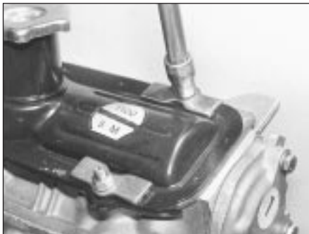
42.26 Tightening a camshaft carrier cover nut
