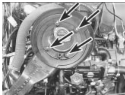
2.11A Air cleaner mounting studs (1116 cc)
