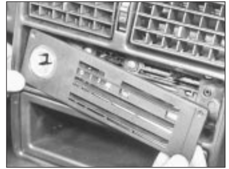
12.6B Removing heater control panel escutcheon
