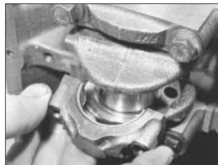
5B.98 Fitting a big-end bearing cap
