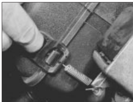
9D.17A Release the air cleaner end cover retaining clips . . .
