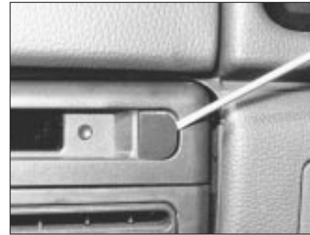
15.62 Prise free the trim covers for access to retaining screws . . .
