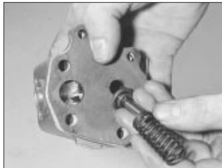
7B.180A Locate pressure relief valve and spring on the intermediate plate
