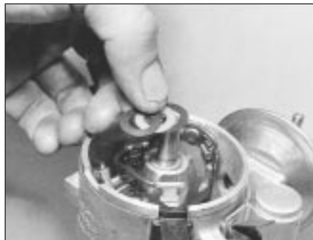
2.22B Washers above contact breaker
